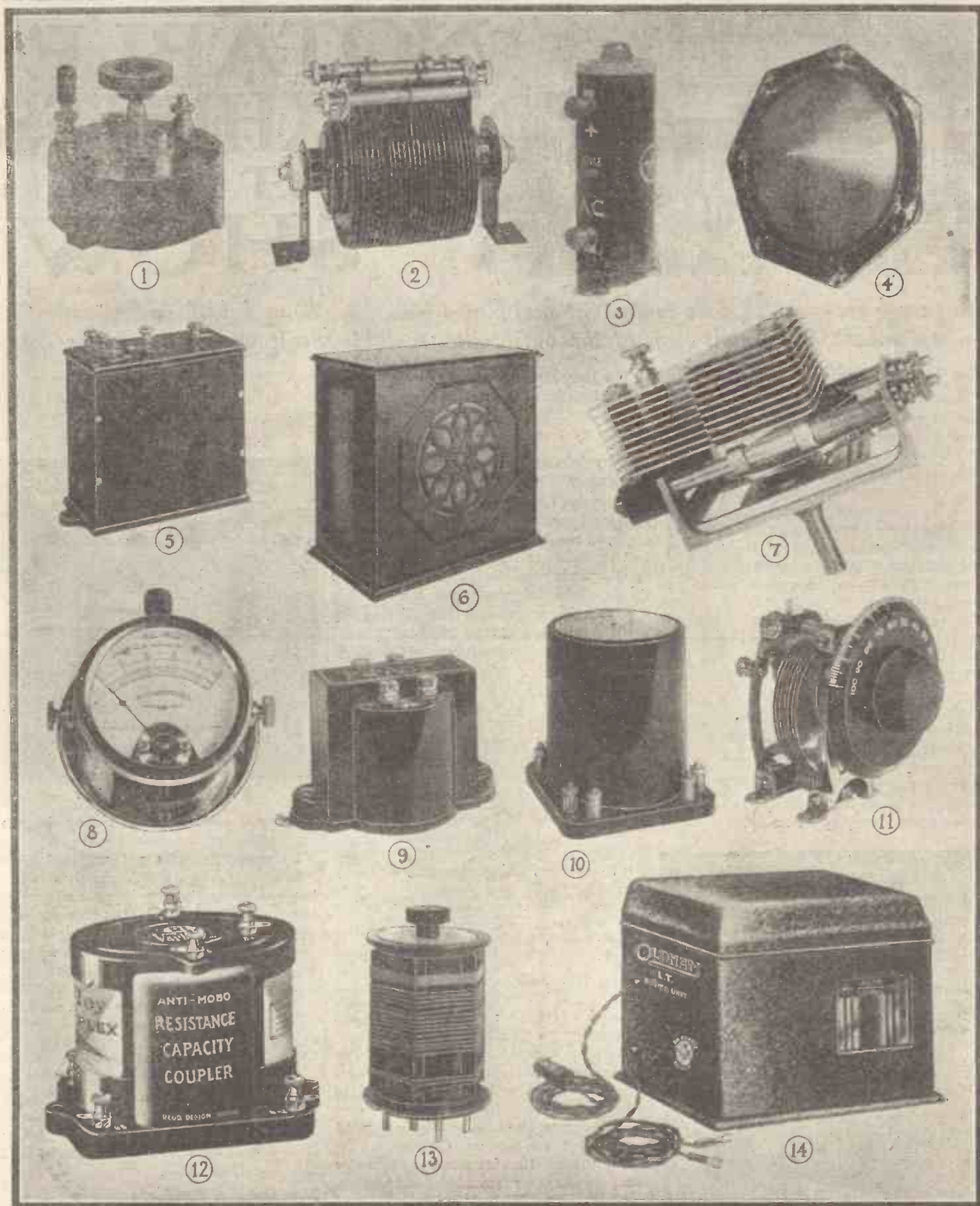
1—Cosmos Elastic Aerial Unit. 2—Westinghouse Metal Rectifier 9 volt 1 amp. type. 3—Westinghouse G.B. 45 volt Rectifier. 4—Phillips loud-speaker. 5—Wearite Anti-mobo. 6—Marconiphone Moving-coil Loud-speaker. 7—Ripaul's Lateral-action Condenser. 8—Hunt's Milliammeter. 9—Igranic Type J Transformer. 10—Formo 2-stage L.F. Unit. 11—Lissen Variable Condenser. 12—R.I. and Varley Resistance-capacity Coupler. 13—Lewcos Short-wave Coll. 14—Oldham L.T. Power Unit.
