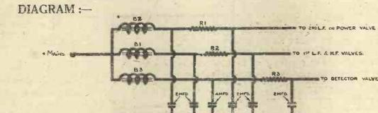
FILTER CIRCUIT FOR A SET CONTAINING H.F. DETECTOR AND TWO L.F. STAGES.
