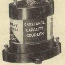
Type A. Suitable for use after Valves with A.C. Resistance (Impedance) of 15,000-40,000 ohms ... 20/-Type B. Suitable for use after Valves with A.C. Resistance (Impedance) of 30,000-100,000 ohms ... 22/6 Illustrated leaflet C14 free on application.
