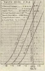
Flg. 6.—Characteristic Curves of Mullard Valves, the P.M.1 L.F. and P.M.2.
