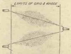
Fig. 7 .- Diagram showing Distribution of Electron Emission.
