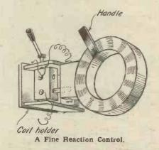
ebonite handle which is fixed to the coil itself. It will be apparent that moving the reaction coil slightly out of the plane parallel to that of the fixed coil will effect smaller variations of coupling than are obtained when the reaction coil is moved bodily away from the fixed coil.
