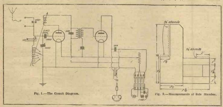
(Lissen T.1); one fixed condenser, .0001 (Dubilier); one fixed condenser, .002 (Dubilier); one fixed condenser, .004 (Dubilier); one fixed condenser (with gridleak clips), .0002 microfarad (Dubilier); one grid leak, 2 megohms (Dubilier); one 1-microfarad Mansbridge condenser; one
