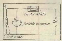
Fig. 1.—Crystal Set Back-of-panel Wiring.
