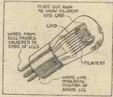
Fig. 10.—Showing General Construction of P.M. Valves.
