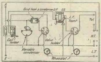
Fig. 3.-Wiring Diagram of Two-valve Set.
