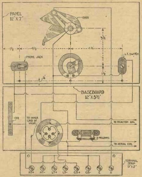
The Developed Wiring Diagram of the Four-electrode One-valver.
