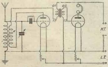
Fig. 4.—Circuit Diagram of Two-valve Set.
