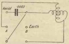
Diagram of Connections for Variometer.
