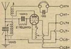
The Four-electrode One-valve Circuit Diagram.
