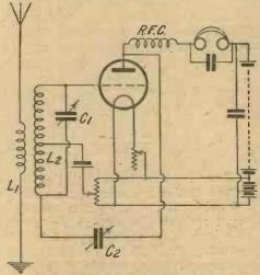
Fig. 2.—One-valver with Anode-bend Rectification.
