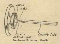
1/4 in. apart. This fork is then soldered centrally on the head of a 6 B.A. bolt. To use this extension arm, two holes 1/4 in. apart must be drilled 1/8 in. deep in an ordinary ebonite knob, such as is usually fitted to a variable condenser. The final fitting arrangements are made clear in the W. G. A.
