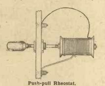
which is made to slide accurately in a brass bush attached to the vertical panel. Above the bush is bolted as springy brass strip, the free end of which engages the winding; below the bush is attached a small bolt carrying a flexible lead which is connected to one end of the winding. The connections are made to the lock-nuts on the two bolts. B. M.
