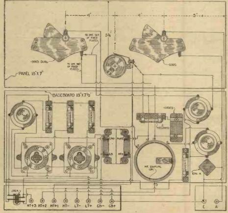
Fig. 3.—Developed Wiring Diagram.
