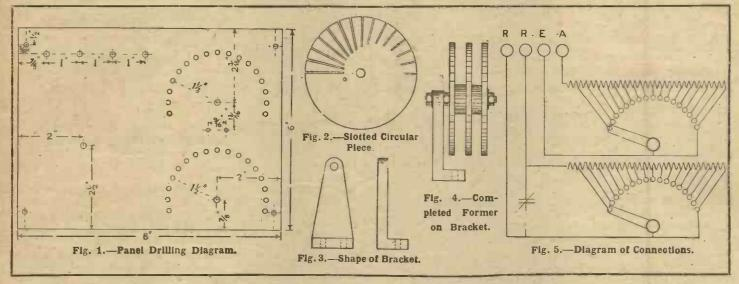
difficulty in construction. The former for the coil windings can be cut with a fret- or hack-saw and finished with a file, no machining being necessary.
