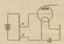
Fig. 3.—Method of Applying Negative Potential to Grid.
