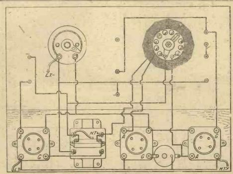
Fig. 3.—Developed Wiring Diagram.
