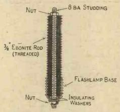
Fig. 1.—Sectional Drawing of Resister.
