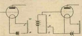
Fig. 1.—Use of Filament Resistance.
