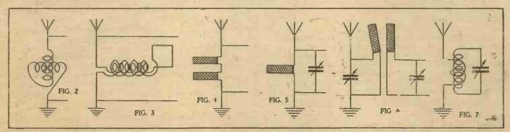
Figs. 2, 3 and 4.—Three Types of Variometers.
