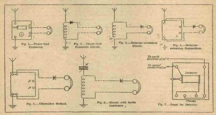
This trouble can be easily overcome. Instead of merely extending the phone leads, as in Figs. 1 and 2, the crystal detector is taken to the distant room next to the phones, as shown in Fig. 3.
