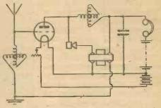
Fig. 7 (left).—Arrangement of Components. Fig. 6 (above).—One-valve Reflex Circuit.
