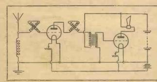
Fig. 3 (right).-Circuit with Frame Aerial.
