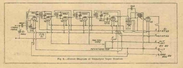
which go to the baseboard; all the others are fed from the L.F. transformer and terminal panel. After wiring, it will be found that before connecting up to the baseboard, the panel will have to be fitted and the filament wires on the baseboard slightly adjusted so as not to short-circuit the two filament rheostats.
