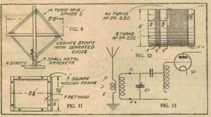
Fig. 8.-Frame Aerial. Fig. 11.-End of Cabinet. Fig. 12.-Inductance for Outside Aerial. Fig. 13 .- Circuit for Outside Aerial.
