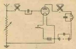
Fig. 2 .- R.A.F. Short-wave Receiver Circuit.
