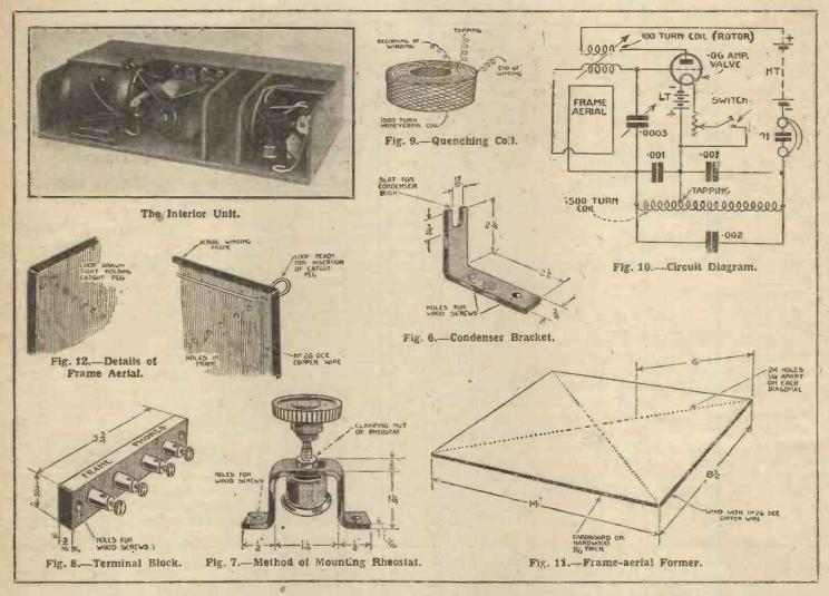
Wiring up, using rubber-covered wire, is carried out as shown in Fig. 10. All joints should be well made, as in carrying the set about there is always a risk of a connection coming unfastened.
