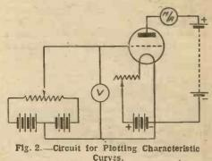
Now a method of overcoming this drawback is to introduce heavy damping into the various circuits, generally by means of positive grid bias. Therefore, by connecting up a potentiometer as shown in the sketch, it is possible to control the grid
