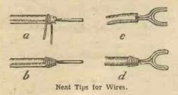
wound with small bare wire to prevent the insulation from unravelling. a and b show the insulation removed from the wire and the neat finished effect. c and d illustrate the method of making a spade tip for connecting to terminals. The latter is a connection that is especially useful when the wire is to be frequently connected and disconnected. F. C. L.
