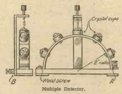
whisker arm are both made of brass strip, the former having a radius of about 2 in. and the latter being about 3 in. up to the bend. By using this, several different types of crystal can be tested without having separate stands. The only terminals used are those marked A and B in the diagrams. F. C.
