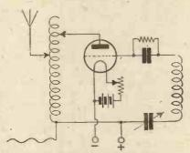
Fig. 28 .- A Circuit with Series Grid Condenser.
