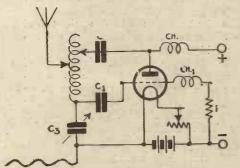
Fig. 32.—The Colpitt's Capacity-coupled Circuit.
