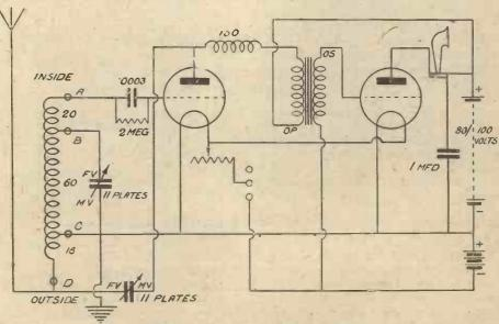
Fig. 1.—Circuit Diagram of Two-valve Reinartz Receiver.
