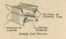
spaced to a distance approximately equal to the diameter of the wire.
