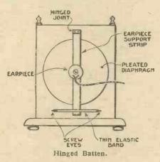
shown in the diagram, and a thin rubber band is placed round the batten to prevent any movement sideways. No pressure should be exerted on the phone, as the weight of this will be found sufficient for good results.
