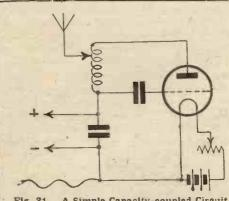
Fig. 31 .- A Simple Capacity-coupled Circuit.
