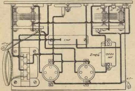
Fig. 3 .- Wiring Diagram of Reinartz Receiver.
