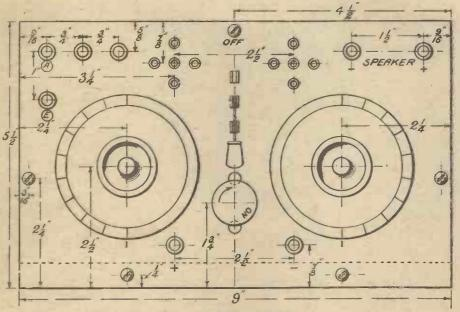
Fig. 2.-Layout of Panel.
