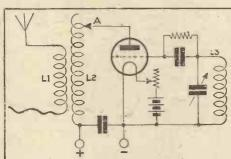
Fig. 27 .- A Simple Form of "Ratio-tap" Circuit.
