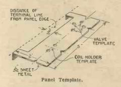
the device is placed with its two lugs against the edges of the ebonite and the lines for the terminals are scribed without the need for making any measurements from the panel edge.
