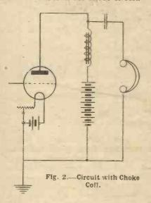
The secondary winding of an ex-W.D. spark coil makes a good choke, as also does the secondary winding of a goodquality intervalve transformer. Many experimenters have on hand an old transformer with a burnt-out primary which can be pressed into service. Regarding the fixed condenser, this may well be an ex-W.D. 2-microfarad Mansbridge pattern, which may be purchased for a small sum from most dealers. The writer has used the arrangement described above for some months with every satisfaction.
