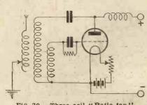
Fig. 30.—Three-coil "Ratio-tap" Circuit.
