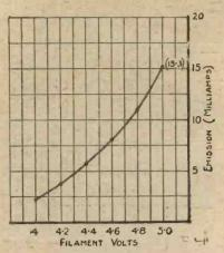
Fig. 1.—Emission Curve (Plate Volts, 50);
