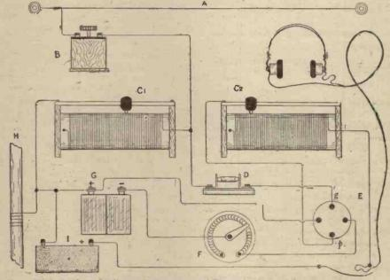
Method of Connecting-up Apparatus for Single-valve Regenerative Receiver.
