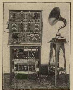
A Five-valve Experimental Receiver constructed from a Peto-Scott Unit Set.
