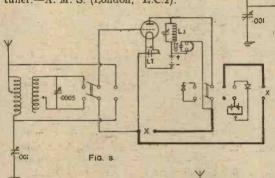
A.—Fig. 1 shows the method of adding a valve detector to this receiver, making use of the "valve" position of the right-hand change-over switch, and the valve terminals on the right-hand side of the panel. This figure refers to the reply to a question on page 858 of AMATEUR WIRELESS, June 23rd. The whole of the circuit within the dotted lines constitutes the valve detector circuit which may be suitably movinted on an
