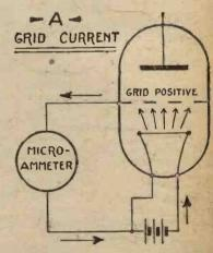
Fig. 4.—Measuring Reverse Grid Current or
