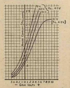
Fig. 3.—Grid-volts and Anode-current Curve.
