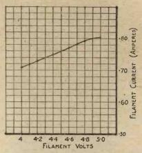
Fig. 2.—Filament-volts and Filament-current Curve.
