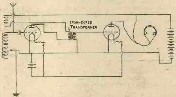
Fig. 4.—Note-magnification Circuit.
