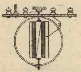
Fig. 1. Section of Complete Variometer.
