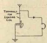
Fig. 3 .- Circuit Diagram of Variometer Receiver.
