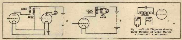
of distortion, and amplification is good. The open core is, theoretically, not so efficient at low frequencies as the closed, but thanks to its design this transformer leaves nothing to be desired. This type can occasionally be purchased secondhand, and if it is offered at a reasonable price it should certainly be snapped up, for it is as handy a piece of apparatus as
