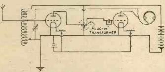
Fig. 2.—Method of Connecting Two Valves with Plug-in Transformer.
