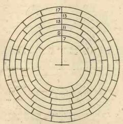
Coil-pin Spacing Diagram.
