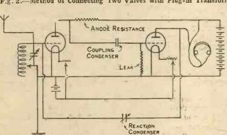
Fig. 5.—Resistance-dapacity Coupling.
