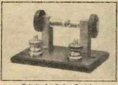
Detector for Broken Crystals
