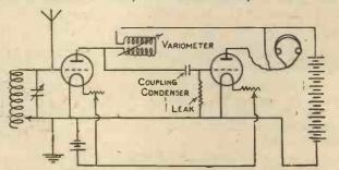
Fig. 3.—Tuned-anode Coupling.
