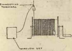
Fig. 3.-Winding Drum and Receiver Connection
