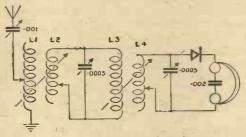
Fig. 14.—A three circuit, or multi-tuner, re-Consists of three separate circuits, each of which is tuned to the incoming wavelength. Two loose couplers can be conveniently used in this circuit in conjunction with three variable condensers whose values are given in the diagram.
