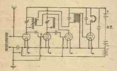
Four-valve Tuned-anode Circuit.
