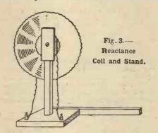
see that the coils are placed so that the windings of all are in the same direction. When this is done the coils have to be joined up in series, that is, the wire left over at the finish of one coil being joined to the commencement of the next. The two outside ends are taken, one to the terminal marked B and the other to No. I contact stud, the joined wires of the remainder being taken to each of the remain-
