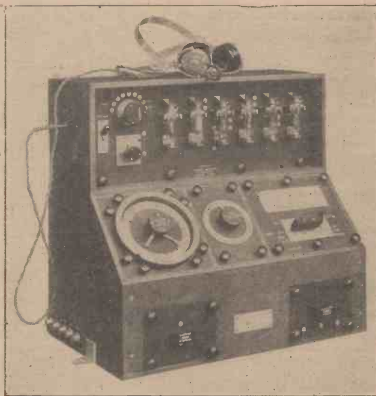
Receiver (including the "Radio-goniometer") Used in Conjunction with the "Balanced Aerial" Directional System.
