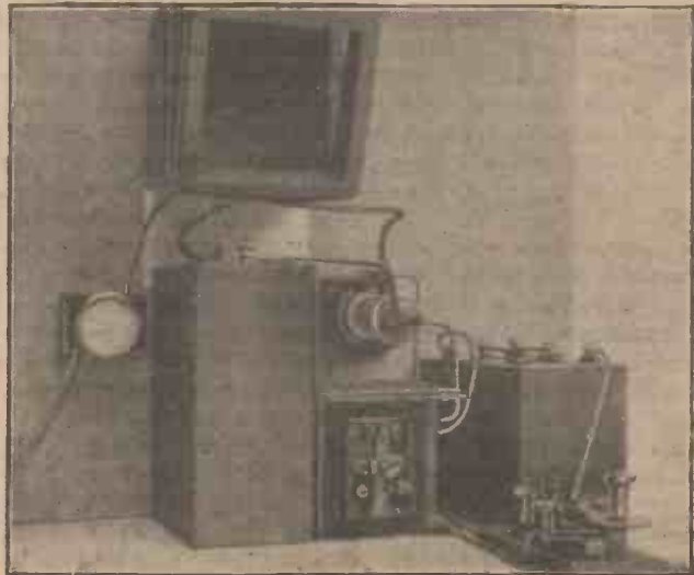
Fig. 1a.—Photograph of Complete Transmitting Set;
