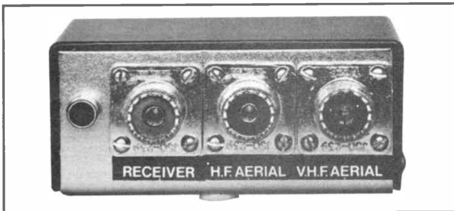
Rear view showing antenna and power supply connectors
