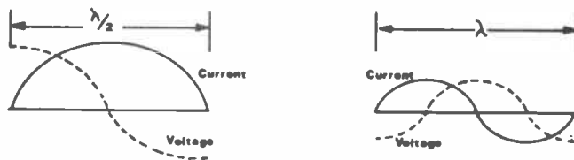
Fig 2 Standing waves on a resonant antenna of \lambda/2 and \lambda .
