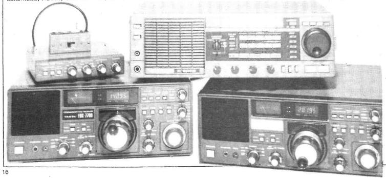
the receiver is muted allowing it to be used with a transmitter. An extension speaker can be interconnected with a 3.5mm jack socket. The set can be used either with normal AC mains or 13v DC, a separate socket being provided for the latter. An accessory socket provides 11v DC, the AGC line, mute output and ground.
