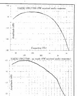
At a glance comparison of the various rigs' performance in terms of FM, SSB received audio response. All tests carried out in January and February this year, and on new equipment.
