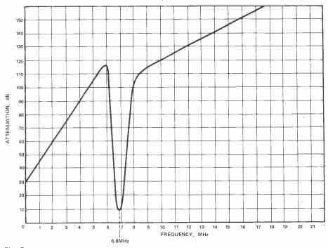
Fig. B Graph showing the attenuation at different frequencies for an antenna buried one metre in silver sand. The Kondratieff Anomaly is clearly shown centring on 6.8MHz.
