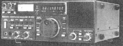
The R70 covers all modes (when the FM option is included), and uses 2CPU-driven VFOs for split frequency working, and has 3 IF frequencies. 70MHz, 9MHz and 455KHz, and a dynamic range of 100dB. It has a built-in mains supply. Other features include input switchability through a pre-amplifier, direct or via an attenuator, selectable tuning steps of 1KHz, 100Hz or 10Hz, adjustable IF bandwidth in 3 steps (455KHz). Noise limiter, switchable
