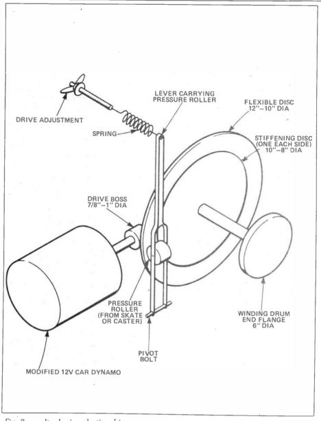
Fig. 2: an ultra basic reduction drive
