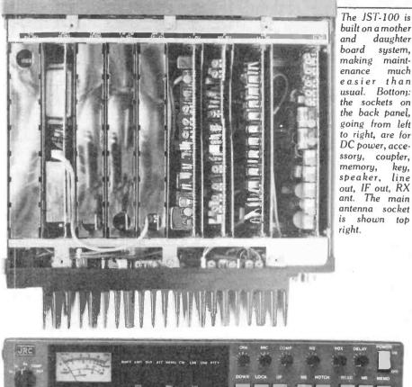
the sockets on the back panel, going from left to right, are for DC power, accessory, coupler, memory, key, speaker, line out, IF out, RX ant. The main antenna socket is shown top right.
