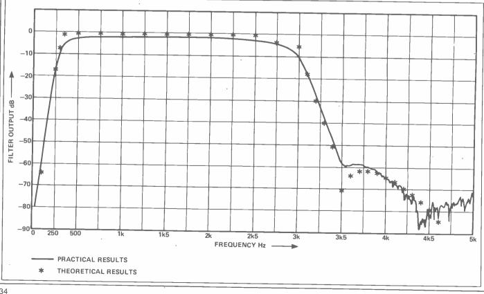
Fig 3: theoretical and practical frequency response curves for the filter. a 1k resistor between the output terminal and earth, and then feeding into a high impedance (say, greater than 10k) audio amplifier.
