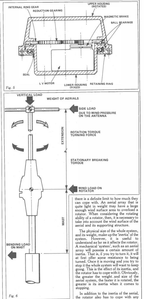
'turning' loads that the wind can generate, such as when the wind strikes one point of the aerial more than others, thus trying to 'weather cock' the aerial.
