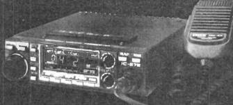
And we thought that the IC25E was small! ICOM have now produced a new and even smaller 25W FM 2 meter mobile the IC27E.
