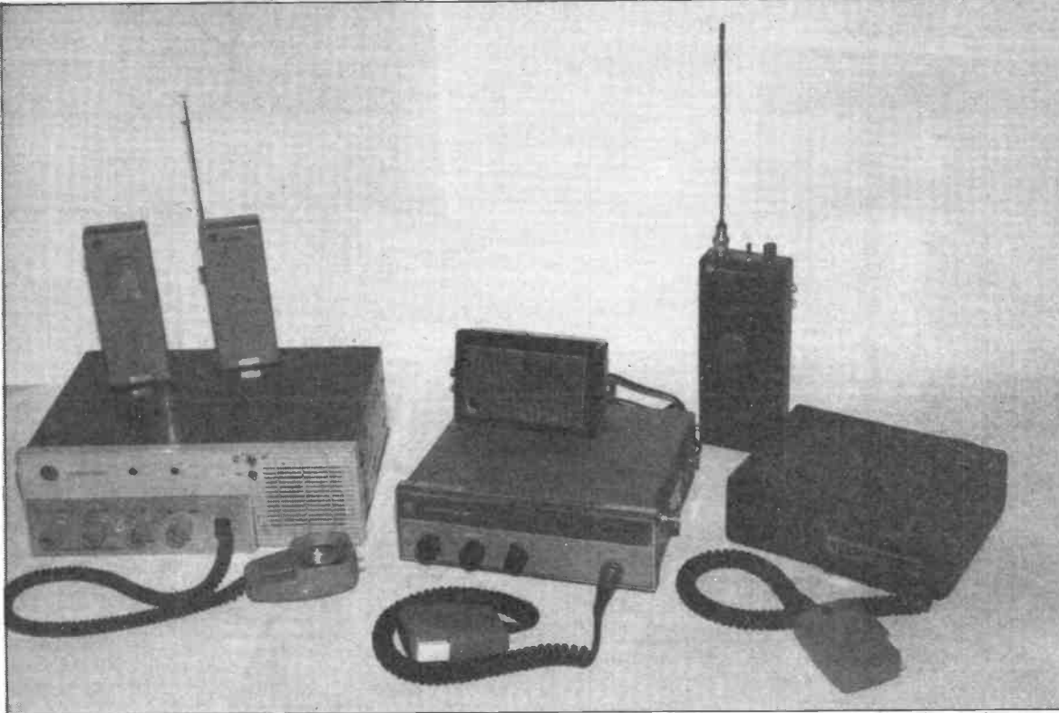
Left: Pye transceivers old and new. From left to right: Cambridge, with Pocketfone PF1 receiver and transmitter on top of it; Westminster; Pocketfone 70; Pilot. Far left: Westminster with portable rechargeable battery and aerial pack. The charger plugs into the Bulgin socket, shown here with the dummy plug inserted. Below: Pilot, the aircraft version of the Motafone.
