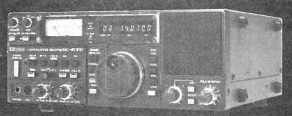
AGC, tunable notch filter, squelch on all modes, RIT, tone control. Tuning LED for FM (discriminator centre indicator). Recorder output, dimmer control. The R-70 also has separate antenna sockets for LW-MW with automatic switching,
