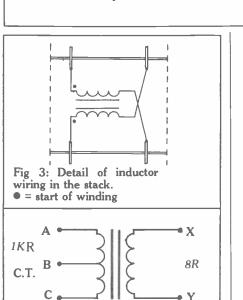
Fig 4: Input/output transformer
