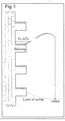
It could also be made up from bamboo with thick wire taped along its length. For single band operation the chimney vertical is best cut to a quarter wavelength at the working frequency and there should be a piece of wire of identical length to run around the edges of the room or under the carpet to serve as the ground plane. Any other metal piping or heating radiators can also serve as additional earthing to supplement the single 'radial'.
