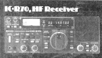
The R-70 covers all modes (when the FM option is included), and uses 2 CPU-driven VFO's for split frequency working, and has 3 IF frequencies: 70MHz, 9MHz and 455KHz, and a dynamic range of 100dB. It has a built-in mains supply.
