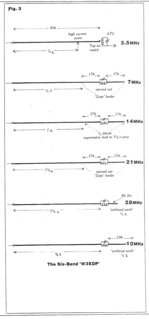
On 7MHz a 17 foot counterpoise is needed. This does not behave as an 'artificial' earth (being only ¼ wavelength long) but acts as half (one leg) of a 17 foot 'Zepp' feed-line to the end of a half wave top! The other half of the feed-line being the first 17 feet of the 85 foot aerial wire we end up with a 'Zepp' with a 68ft top. Although the feed wires are well separated they still behave as an open wire line of high impedance but of course will radiate to some degree.
