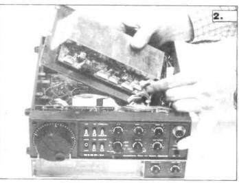
2. Remove power supply assembly by removing fixing screws. Disconnect multipole connector and put assembly to one sidc.
