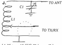
L1 35 turns 16 SUG 2" former 4" long tapped 5 turns up C1 500pf broadcast type variable.
