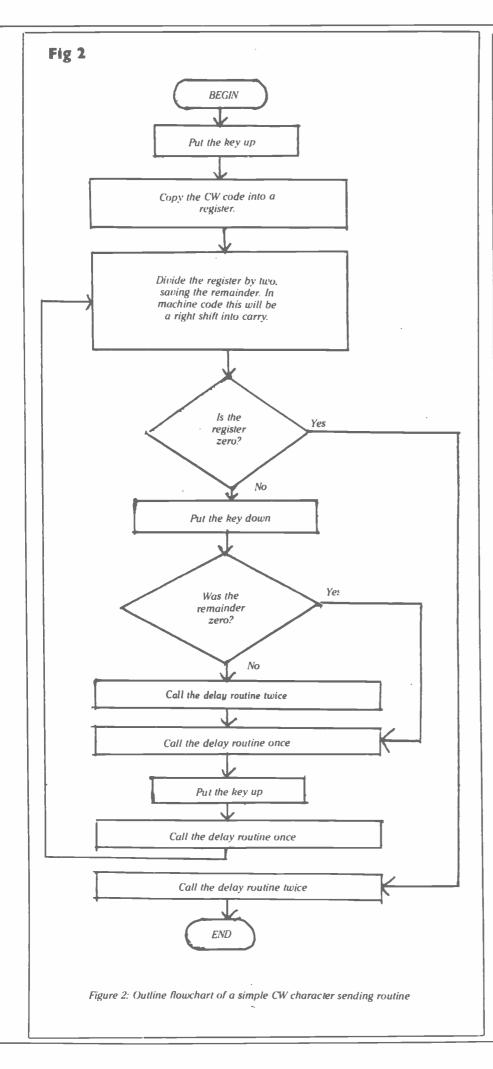
When you get your Morse sending program going you will probably want to calibrate it. The easiest figure to remember is that when the basic time period (the "keydown" time for a dot) is a tenth of a second the speed is exactly 12 words per minute. For higher speeds the dot length is proportionately shorter, and vice-versa.
