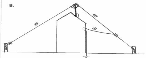
A method of fabricating an inverted vee aerial (quarter wave) over a house. This does work and can be fitted into small gardens. It is, however, much inferior to the half wave. If open to an upstairs shack the length of conductor to earth affects performance and increases noise pick up (live should be insulated from all anchor points). (The aerial can be bent round to suit individual site).
