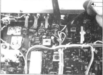
Remove carefully the wire soldered between antenna socket and main pcb. Solder (as shown) red-coded coaxial cable to antenna socket, braid to associated solder tag.
