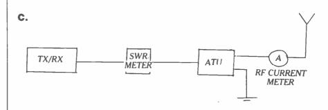
A method of connecting rig to end fed, current fed or other low impedance fed aerial. The SWR meter ensures a good match between rig and ATV. With such aerials (e.g. 132' wire) the object is to get as much RF current as possible indicated in the RF ammeter. The reading on the ammeter will depend upon aerial length and earth efficiency. Add radiaes or earth spikes until a greater reading cannot be obtained.
