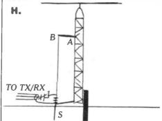
Gamma match feed of earthed tower. Correct impedance obtained by moving point A up and down tower, and by making A to B longer or shorter. S earth spike connected to base of tower. Use of quarter wove radials parallel to ground will improve radiation efficiency.
