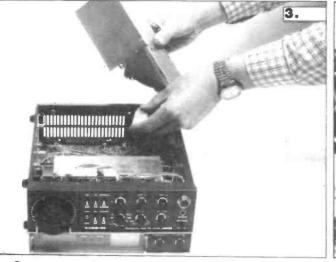
Remove synthesiser assembly. Do NOT forget fixing screw located through main pcb. Note positions of connectors and remove. Lift assembly clear.
