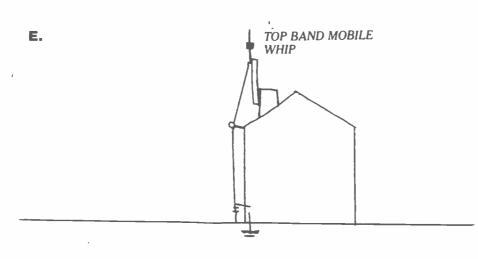
An old or redundant mobile whip can be used by connecting its base to an insulated (non metalic) pole attached to chimney etc. The base is connected to wire down lead and taken via a stand off insulator to the shack. The whip and the downhead will act as the aerial, but the conductor below the loading coil does the work. Such a system can be turned by using a series tuned ATV or a series inductor.
