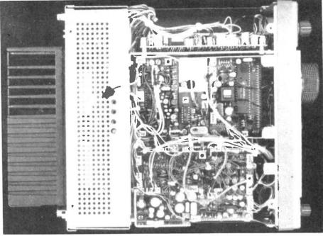
View of FT77 with bottom cover missing. Speaker is mounted on top, which could prove a problem to mobile operators.
