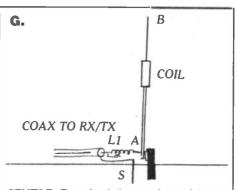
CENTRE: Front loaded vertical aerial from A to loading coil is 20' dural tube (length not critical). Coil should be wound on as greater diameter forms as practical with as thick wire as possible. From coil to B is 9' to 12' dural tube or tank whip. L1 variable induction (roller coil).
