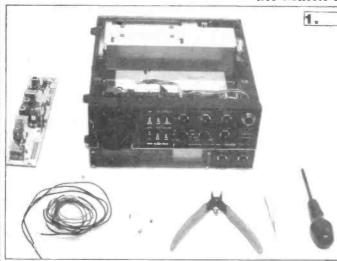
**1**. Top and bottom covers have been removed from the transceiver. Mutek board (left) is poised for action with tools for the job.
