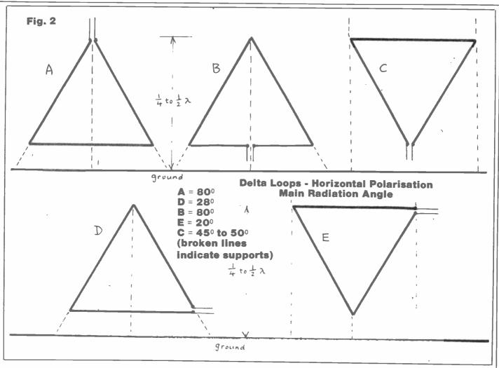
either! The type of wire used (single, stranded, bare or plastic covered) the insulation at the support points and the proximity of trees and other objects will have a greater impact upon resonant length and the difference between the two calculations.
