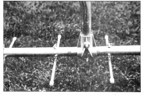
Anyway, the other relevent figures for the 18-element Parabeam suggest a front-to-back ratio of 18dB and a 3dB beamwidth (which tells you who sharp the thing is, in effect) of 25 degrees. The boom length of the beast is 2.8 metres.
