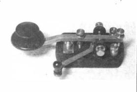
MorseMatic device and on the right is one of the simplest coilsprung keys. Left: One of the oriainals.
