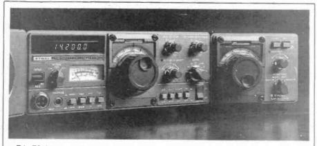
Trio TS130S is a sort of transistorised variant of the TS530; the 130V is a lower-power version. Good middle-class radio for the newcomer.
