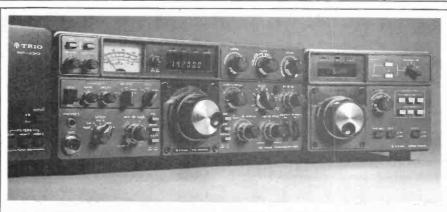
*Trio* TS830S — a typical upper-middle class HF SSB machine, developed from the very successful TS820. Very reliable and versatile; lots of facilities, excellent transmit strip but receiver lets the side down a bit . . . however, a pretty rig all in all.
