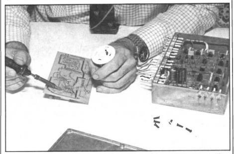
Above: Soldering components on to a printed circuit board. Practice soldering and get it off to a tee before you work on the PCB. Below: Basic equipment needed in order to build your own radio, or carry out proper maintenance: screwdrivers, pliers and cutters, drills, soldering iron, and hacksaw.
