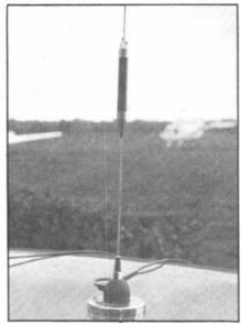
Typical mag-mount mobile 70cm vertical antenna — note the loading coil partway up the rod.
