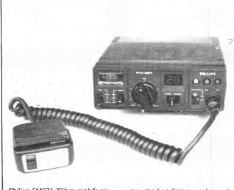
Philips FM321 70°cm mobile rig — a very good performer and easy to use in the car, this machine will give 40 channels on 432 MHz and can be used for repeater working.
