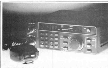
Trio TR7800 FM mobile 144 MHz rig, featuring selection of frequencies via a "keypad" and the ability to re-tune via switches on the microphone; an extremely good performer, with full repeater and simplex facilities in a compact box.
