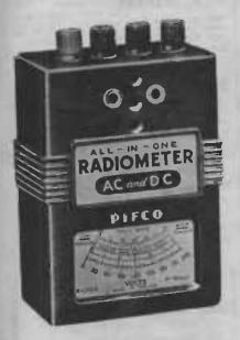
Pifco goes straight to the heart of the trouble, testing sets and components with equal ease and speed. Any radio set can be tested, either A.C. or D.C. Mains or Battery operated. Solidly constructed in a fine bakelite case 4in. x 22in. overall. The Pifco Radiometer has readings for high and low voltage, milliamperes, ohms, continuity test, etc.
