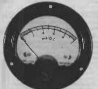
0-1 M.A. Moving Coil D.C. Meters. 1000 ohms per voit. Internal resistance 60 ohms. DE JUR (U.S.A.), 2§in. Round Scele, 3§in. Outside Diameter. Cat. No. AM15
