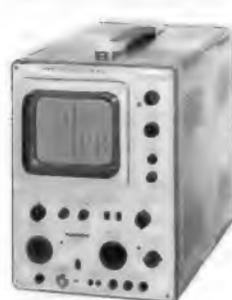
**Trigger-Oszillograph HM 312**
