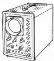
HF-Oszillograf GM 5601 X: 0...300 kHz, 1 Vss/cm Y: 0...5 MHz, 100 mVss/cm
