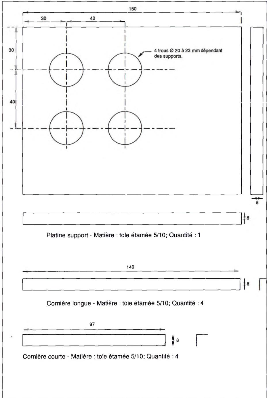
Fig. 21— Platine support des tubes.
