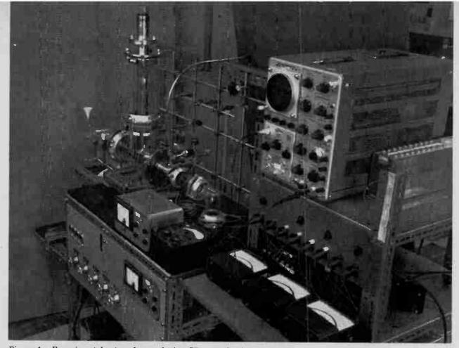
Figure 1. Experimental set-up for producing SF6 negative ions for charge neutralized ion engine.
