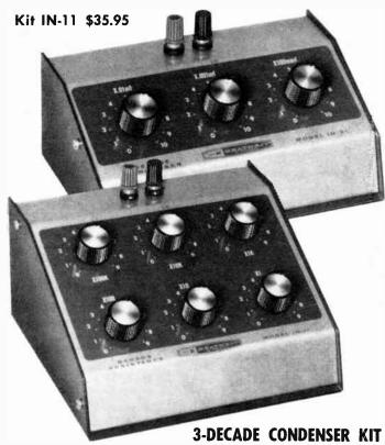
Use this in any application requiring precision capacitor values. Provides capacitor values from 100 mmfd to 0.111 mfd in 100 mmf steps. Capacitors are precision 1% silver mica types rated at 350 volts DC, continuous; 500 volts DC, intermittent; and 1000 volts DC test. Switches are high quality low-loss ceramic wafer types with positive detent action. 3 lbs.
