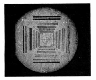
This is an actual size portrait of an NBS resolution chart taken at 0.1 microsecond with an Abtronics electronics framing camera
