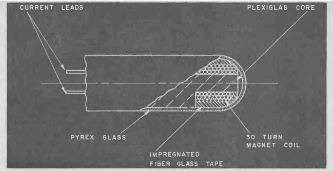
Figure 3. Diagram showing a hemispherical-nosed hypersonic flow model which contains a coil for generating a magnetic field.
