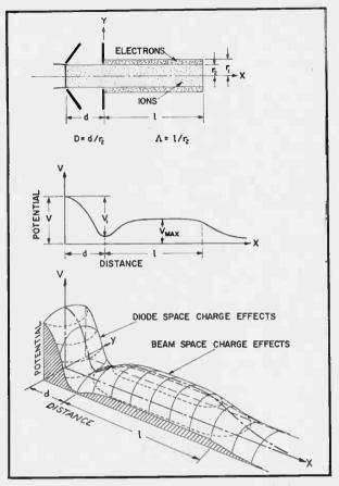
Figure 4. Diagram showing potential variation contours in the exhaust of an ionic rocket.
