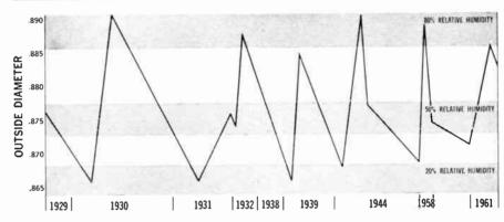
Long term test of fibre, which has been going on since 1929, shows that fibre still responds to wide humidity changes in the same way it did when test began. Predictable changes in dimension occur when fibre tubing is subjected to extremes of humidity. Tests such as these prove that there is no change in Vulcanized Fibre characteristics over long periods of time.
