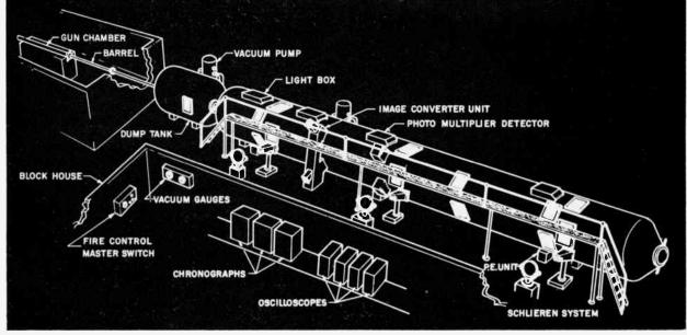
Figure 1. Layout and instrumentation of a hypervelocity range facility.
