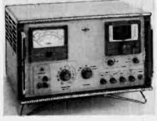
Electro instruments inc. Model 4010 Digital Voltmeter, 1 millivolt to 999.9 volts DC automatic ranging and polarity highly reliable solid state circuitry accuracy  $\pm$  1 digit +.002%/degree C.
