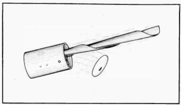
Figure 5. The self-extending "Jack-in the-box" sideejecting design.
