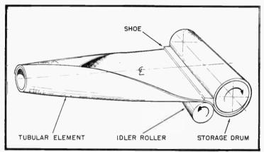
Figure 4. Design using the principle of radial lead-off using curved shoe idler roller.
