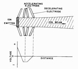
Figure 3b. The "accel-decel" ion-engine structure and diagram showing voltage distribution.
