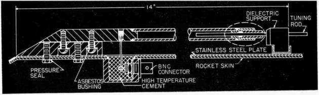
Figure 5. Diagram of the NRC designed rocket antenna.
