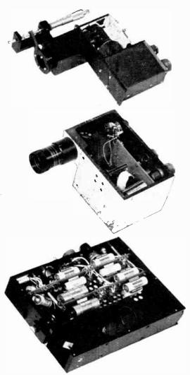
Figure 5. (top-a) ultra-violet and visible measuring module (De Havilland Aircraft Co.) (center-b) ultraviolet module (Perkin Elmer Corp.) (bottom-c) Infrared measuring module (Perkin Elmer Corp.).
