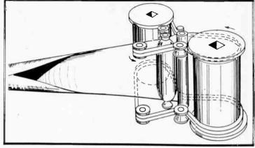
Figure 2. Diagram showing principle of tube extension for designs employing spring or rubber belts.
