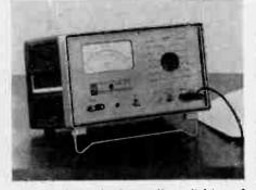
Sierra Electronic Corporation, division of Philco Corporation, Model 127A Solid State Selective Voltmeter, Covers 2-350 Kc/s, -80to +22 DBM, accuracy  $\pm 1$  db, built-in crystal calibrator, rechargeable battery, light and portable.
