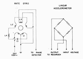
Figure 2. (above) Diagram of helmet gyro and linear accelerometer. Figure 3. (below) Circuit diagram of the phase sensitive detector.
