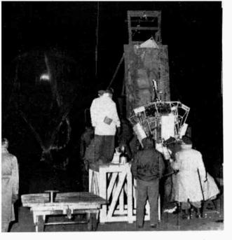
Figure 4. (left) Balloon being filled with helium. Radiometer instrumented gondola is mounted on the launching deck of truck.
