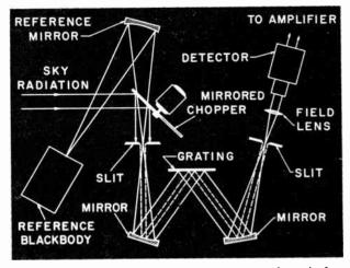
Figure 8. Arrangement of spectrometer for airglow experiments.
