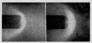
Figure 4. (left) Flow distribution without a magnetic field. (right) Flow with a magnetic field. Note that hot plasma is pushed away from the model thereby reducing heat transfer from the gas.
