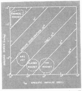
Figure 2. Performance regions in terms of specific power and impulse for various propulsion systems.
