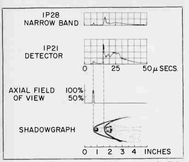
Figure 7. Diagram showing interpretation of radiation detector signals.
