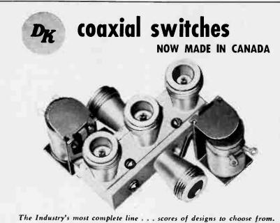
DK Coaxial Switches combine rugged-ness with the highest standards of precision: • Spring-leaf switching blades • Gold-plated silver contacts • Low insertion loss and high isola-tion • Low VSWR (1.3 at 4,000 mc, for example) • Proven mechanical life of 1-ntillion cycles minimum when oper-
