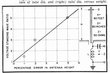
Figure 7. Relationship between mast height mis-match and VSWR for the tubular antenna.
