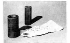
While many materials deteriorate over the years, Vulcanized Fibre maintains its essential properties for decades. Note how the linen tag attached to Fibre tube samples in 1929 shows age, but Fibre tubes look and act as they did 32 years ago.
