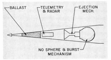
Figure 6. Layout of Nitric Oxide (NO) seeding nosecone.
