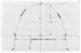
Figure 4. Diagram showing the computation of peak altitude.
