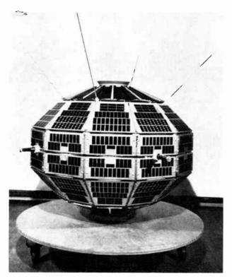
Figure 4. Photograph of the S-27 "Top-side Sounder" satellite.
