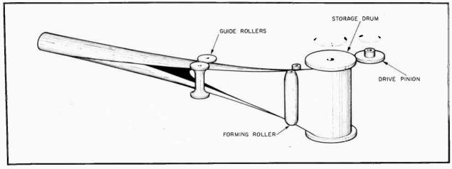
Figure 1. Diagram showing basic principle of operation of the extensible tube.
