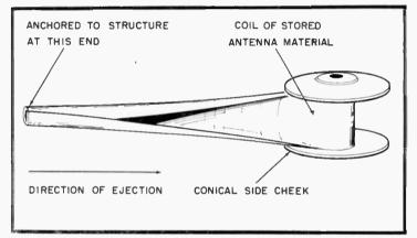
Figure 3. Design employing conical drum cheeks to provide constraint for un-winding strip.
