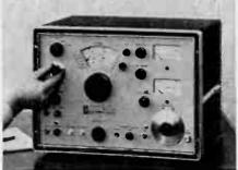
Borg-Warner Controls Model G-201 RF Signal Generator 10 to 420 Mc., 0.1 microyolt to 0.5 volt output into 50 ohms.  $\frac{1}{2}$ % frequency calibration plus built-in crystal calibrator.
