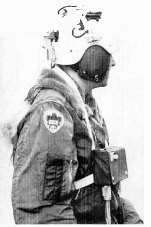
Figure 1. The instrumented helmet for measuring linear and angular accelerations.
