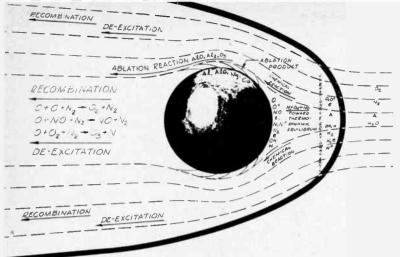
Figure 2. Diagram showing the various processes occurring in the luminous volume surrounding hypersonic bodies.
