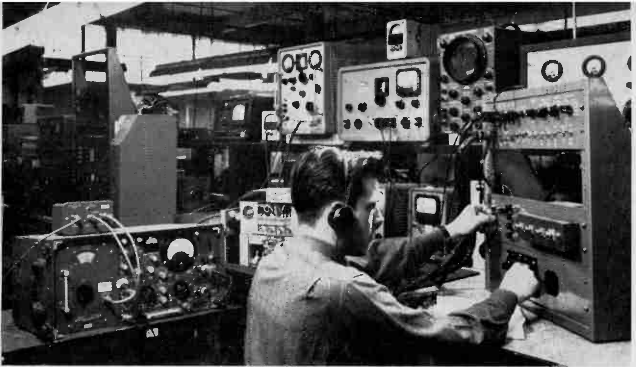
Figure 7. Engineering technician J. Erbersole checks out Collins type 618-W transceiver in elaborately equipped development laboratory.
