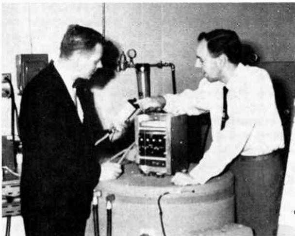
Figure 9. Engineering technician T. J. May (right) of the development department explains to the writer a design feature on transceiver control box just before vibration test on force generator in foreground.
