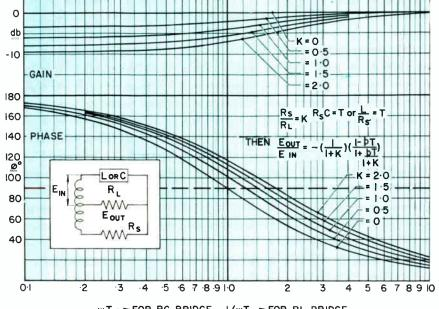
wT -- FOR RC BRIDGE , I/wT -- FOR RL BRIDGE
