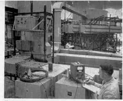
Fig. 3. Being tested (in background) is the high-speed scanning switch housed in large tank. Switch handles multi-megawatt pulses and milli-micro-microwatt return signals.
