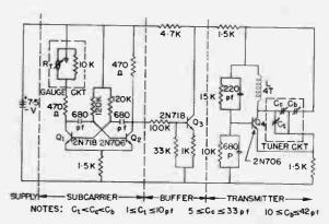
Fig. 7. Circuit diagram of modified temperature telemetering system.
