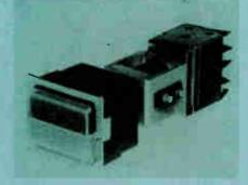
ing. Switch may be depressed and held in Ing. Switch may be depressed and held in able with momentary action and alternate action. Circuiting is 2 pole or 4 pole, 5 amps resistive to 250 AC. Four lamps illuminate the display panel which acts as a button for operating switches. Burgess Micro Switch, 5 Brooklyn Ave., Toronto 8, Ont.
