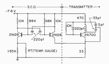
Fig. 4. Circuit diagram of 'high-g' temperature measuring telemetering system.
