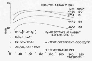
Fig. 8. Normalised temperature telemetering results.
