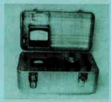
to record observations of inclination, declination, total intensity, orthogonal compo-nent intensity and time variation. Absolute intensity range is 0 to 100,000 gammas; the frequency response of the device is  $0 \cdot 1$  cycle per second.
