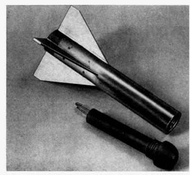
Fig. 10. Photograph of a four fin dart and telemetering package used for stability measurements.
