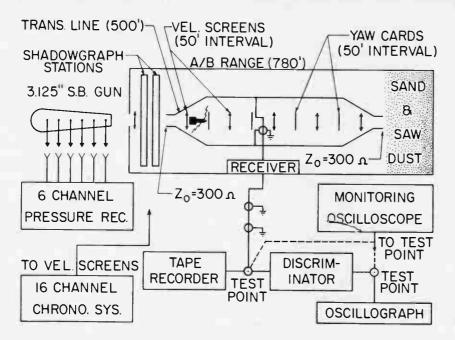
Fig. 6. Block diagram showing layout of high "g" telemetering instrumentation.
