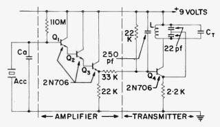
Fig. 9. Circuit diagram of single channel yaw measurement telemetering system.
