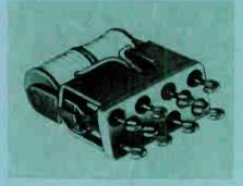
Type F. The relay withstands exposure to Type F. The relay winstands exposure to even more severe environmental extremes, provides the "memory" of a latching device, and may be operated with relatively low power input. Two permanent magnets provide latching forces which hold the contacts in either of two stable positions. C. P. Clare Canada Ltd., 840 Caledonia Road, Toronto 9, Ont.
