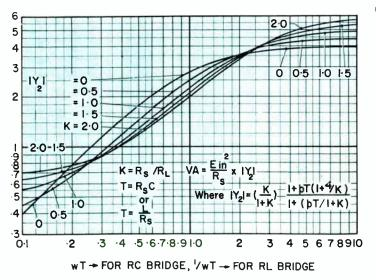
FIG. 2 PHASE SHIFTER IMPEDANCE FUNCTION
