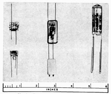
Fig. 2. Illustrating the steps in the production of a telemetering unit.
