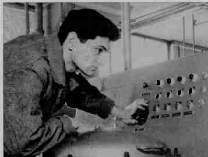
Production process for Rhenium-Tungsten alloy at Chase Brass & Copper Co., Connecticut, is demonstrated as the operator adjusts the power input for the vacuum furnace where Rhenium-Tungsten is sintered at 2500°C and at pressures of .02 microns.
