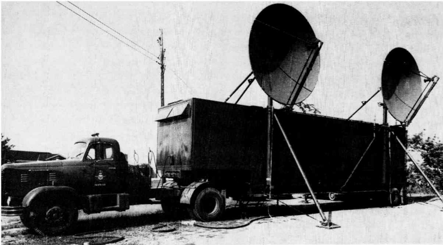
General exterior view of the transportable micro-scatter equipment showing the trailer mounted antennae
