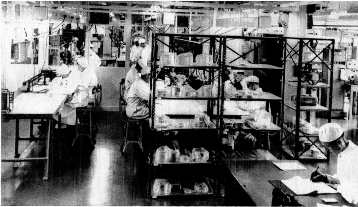
The special area of the Standard Telephones and Cables Ltd. works at North Woolwich, London, England, where the repeaters for the round-the-world Commonwealth telephone cables are being made in conditions of air purity.
