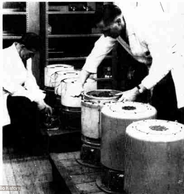
When scientists launch a rocket, they must be confident that its instruments and control mechanisms will withstand the stress of acceleration. E.M.I. Electronics Ltd. new Vibrator Type EMV 100A, which has a frequency range of 1-20,000 cps. is used to pre-test the delicate mechanisms employed for missile control.
