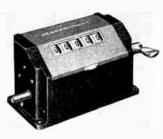
This counter has one set of wheels which are preset to any figure within the capacity of the counter by depressing the reset lever, raising the cover, and turning. The counter subtracts from the preset number to "00000", when a knock-off lever actuates an electrical switch. To reset, just press the reset lever, and counter returns instantly to preset figure. For Mechanical Control, counter actuates a mechanical lever instead of electrical switch. Speeds: 6000 rpm or 8000 counts per minute.
