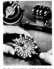
Such connectors (also known as quick-disconnect terminals) are produced by a number of elec-trical hardware manufacturers. Automatic machinery is available to fasten these connectors to the leads at high speed thereby offer-ing important time savings. In use, the "female" connector is pushed onto, and slides over, the tab terminal.
