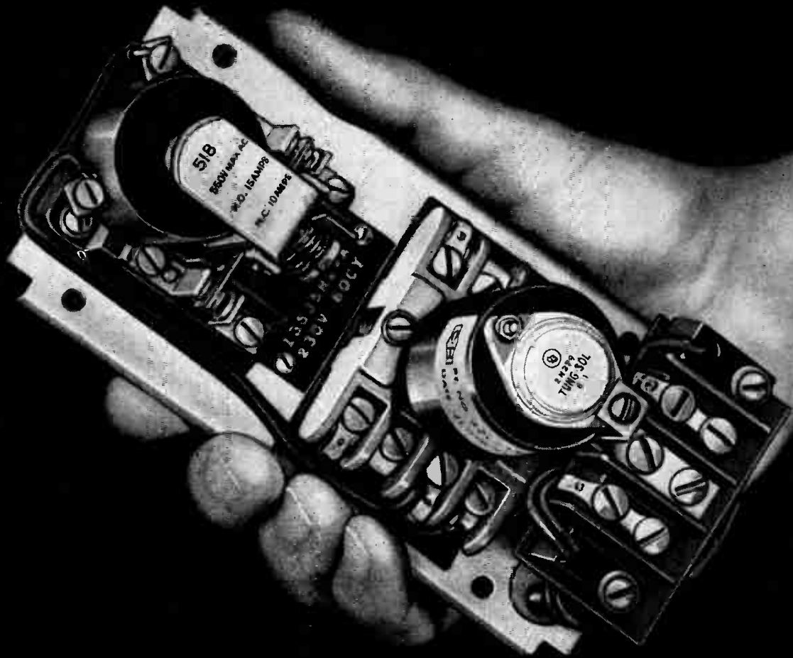
Cutler-Hammer's new sensitive, heavy-duty transistorized relay. The Tung-Sol germanium transistor, power type 2N3790, is at the center of the plug-in module, electronic heart of the relay.
