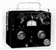
One important feature of the Type 1650-A is Orthonull, an exclusive new mechanical-ganging device which facilitates measure-ment of low-Q inductors (or high-D capa-citors). Orthonull adds convenience and accuracy and makes easy many low-Q measurements that are practically impos-sible on other impedance bridges sible on other impedance bridges.
