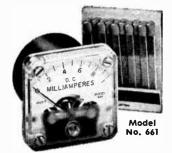
New series for limited space installations. Front opening — 11/2" class — 2% accuracy — standard mounting dimensions — front zero adjustment. In DC ranges from 100 micro-amps; and self-contained rectifier types, VU, and voltmeters up to 300 v.
