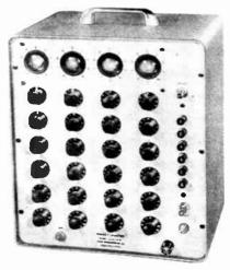
Specifications of Freed's new Preset Counter, Type 2020-4-6 include a maximum 4 digit count of 9,999, operated at counting speeds of 4,000 per second, and presets one through six. Various inputs supplied include Photocell, Switch Closure and Pulse. Output is a Relay DPDT-5 Amp. Contacts, with a 105-125, 50-60 cycles power supply. Dimensions for Type 2020-4-6 Preset Counters are 11 x 13 x 85%" deep. Complete unit weighs 19½ lbs.
