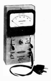
The unit provides an easy-to-read sensitive 50 microampere movement mounted in a sturdy case, is entirely self-contained, and requires no external power connection.
