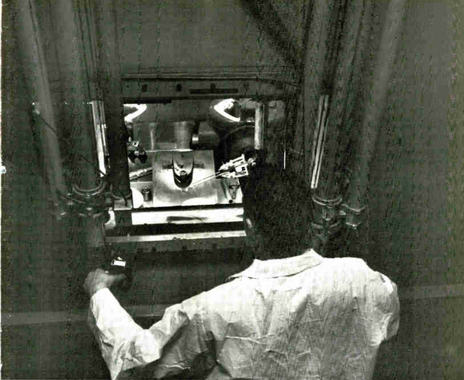
Mechanical hands encapsulate Cobalt 60 (description page 5)
