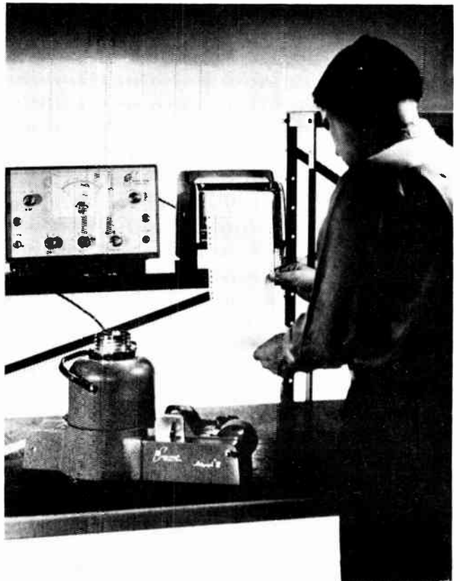
● Strip Foil Analyzer is used to plot induced radioactivity of foils placed in reactor. Strip foils activated in reactor are drawn automatically past Geiger counter in analyzer. Recording shows exponential decrease in activity along radius of uranium lattice.
