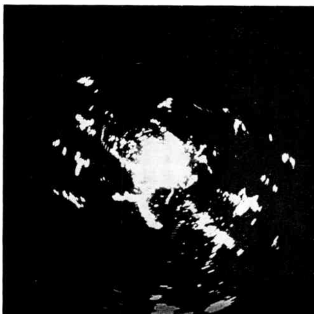
● The Diversity Radar scope picture without Moving Target Indicator equipment.
