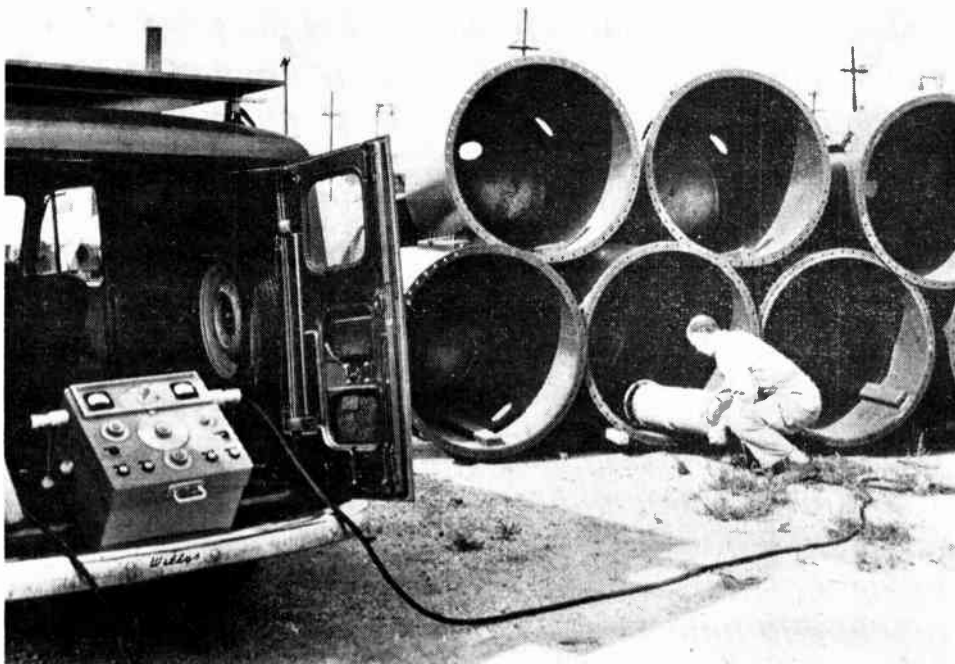
● The OX-175 with control on back of truck. Head is being inserted in pressure vessel preparatory to taking radiography in the field.
