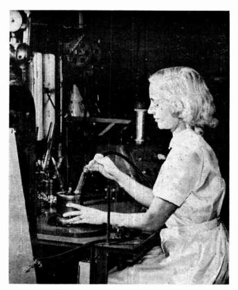
Using Leak Detector to check special-purpose vacuum tubes at Farnsworth Electronics, Fort Wayne, Ind.
