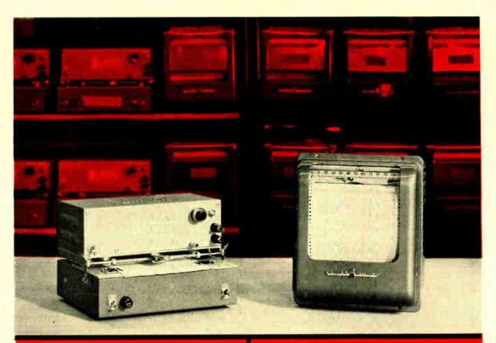
Varian G-10 — Partable for laboratory or benchuse where chart accessibility is of prime importance. Base price \$340. Varian G-11—For panel, rack or portable uses designed for DEM, lab or field for long-term maniforing. Base price \$470.
