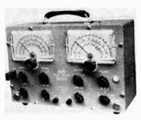
An internal, crystal controlled 4.5 Mc. An internal, crystal controlled 4.5 Mc. oscillator is provided for accurate alignment of Sound I.F. and demodulator circuits. Please note that the Marker Frequency Range of the SMG-57 extends down to 3 Mc., thus allowing the instrument to be used to align F.M. receiver I.F. at 10.7 Mc., as well as providing an option of marker or crystal oscillator at 4.5 Mc.
