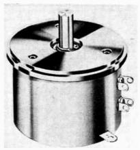
For dependable performance and precise mechanical conformity, stainless steel ball bearings are used, and critical machined surfaces in the housing are turned in one setup. As many as 14 taps can be added during manufacture. Two-gang units are
