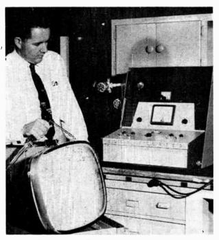
• Using the new CEC Type 24-210 Leak Detector to check leaks in a TV receiving tube.
