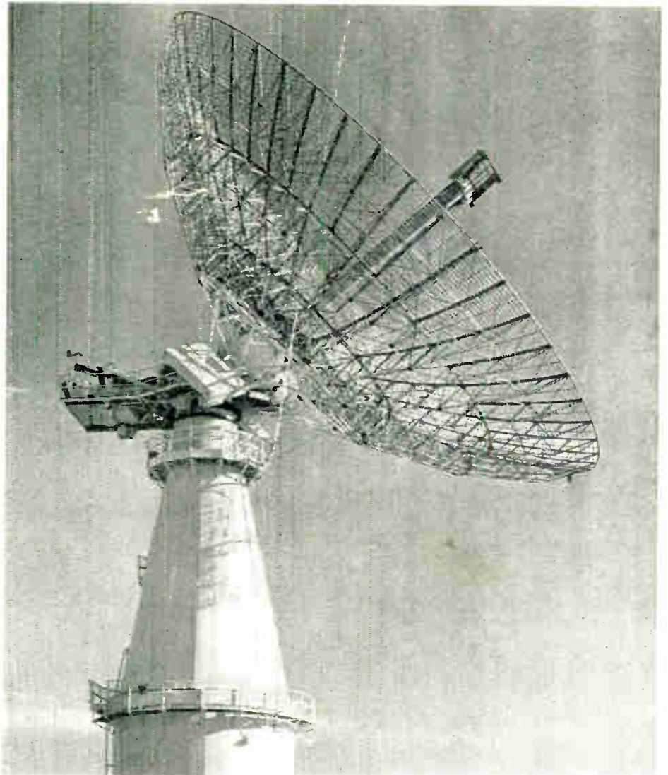
Experimental High-Power Long-Range Radar Installation Developed By Massachusetts Institute Of Technology Lincoln Laboratory.
