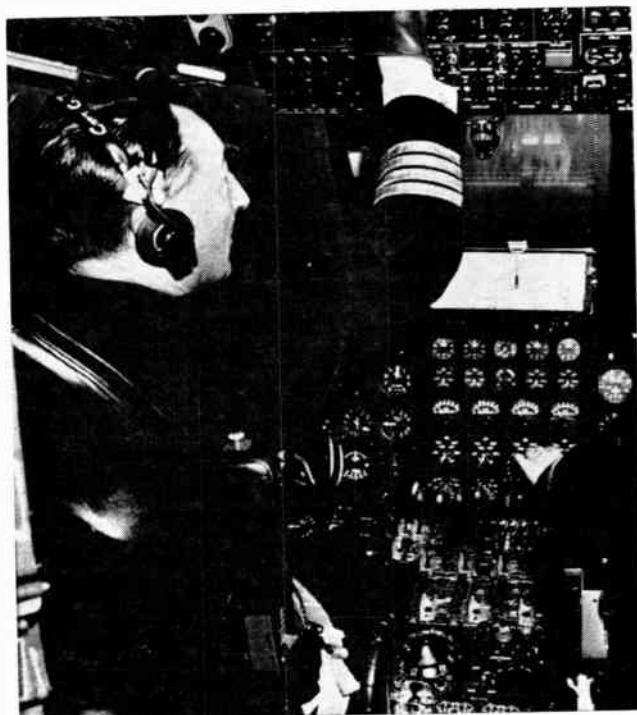
● The "flight log" which interprets continuous signals from the ground stations to give immediate course and position information is seen in the center of this photograph.
