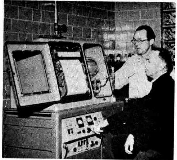
● Operating a CEC Process-Monitor Mass Spectrometer at the Commercial Solvents Corporation, Sterlington, La.
