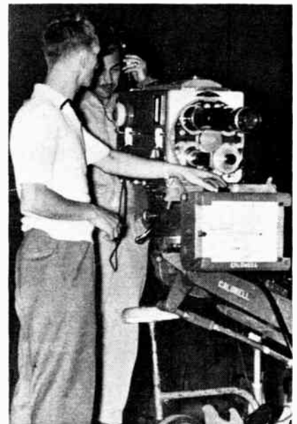
● Photograph shows one of the Pye Image Orthicon studio cameras with TelePrompTer equipment attached which was used to shoot Canada's biggest closed-circuit TV hookup.
