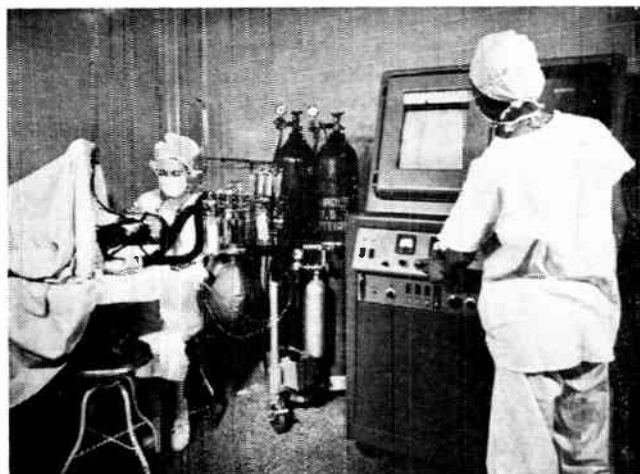
● A CEC Process-Monitor Mass Spectrometer in use as anaesthesia control instrument during surgery at the City of Hope Medical Center.
