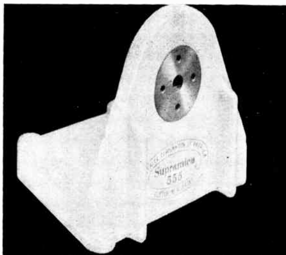
● Massive parts with good physical strength like this tube mounting bracket for guided missile use can be molded from ceramoplastic. The bracket shown measures about six inches across, and weighs several pounds.
