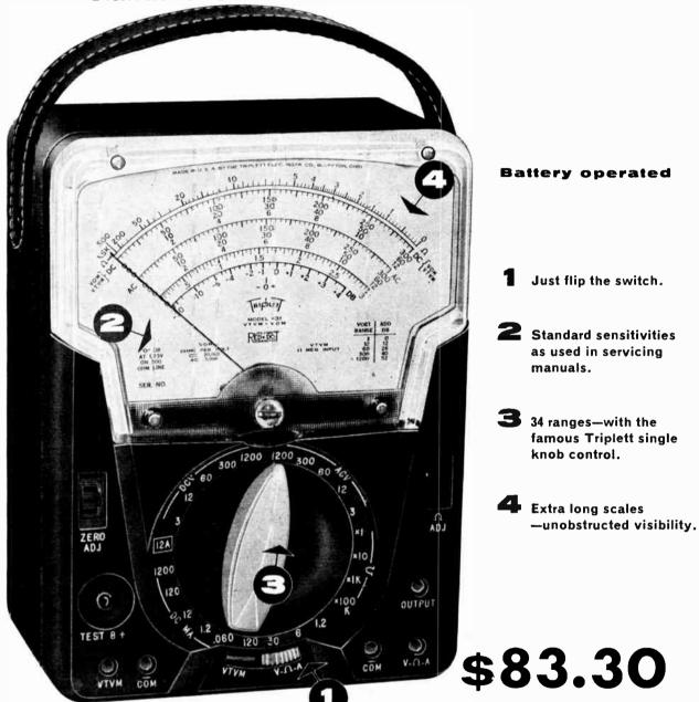
By using the Volt-Ohm-Mil-Ammeter for all general testing (90% of your testing) and the Vacuum Tube Voltmeter only when you need it, you have the advantage of a VTVM with extremely long battery life. Batteries are used only about one-tenth as much as in the ordinary battery-operated VTVM. Features: Ohms, 0-1500-15,000 (6.8-68 center scale. First division is 0.1 ohm.) Megohms: 0-1.5-150 (6,800-680,000 ohms center scale.) Galvanometer center mark "-0+" for discriminator alignment.
