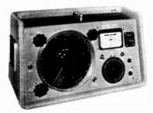
sured at DC. The instrument is entirely self-contained having its own dual-frequency oscillator and detector. All measurements are made directly in the units concerned and no multiplying factor has to be taken into account. Bridge balance is meterindicated in all cases.
