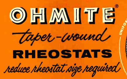
**Tapering the wire size** to match the current carried permits greater capacity in a smaller unit!
