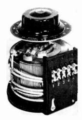
from 0-135 volts. Rated current is 6 amps at 400 c.p.s. 5.5 amps at 1200 c.p.s. Magnetizing current remains less than 50 ma. Load loss is kept to an ultimate minimum — 3 watts at 400 c.p.s. 1.5 watts at 1200 c.p.s. Canadian Electric Resistors Ltd., Curity Avenue, Toronto 16, Ontario.
