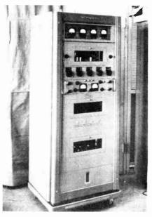
Unit construction is employed so that various channel combinations are obtainable. A modern keying circuit permits keying speeds of up to 600 w.p.m., while the equipment is also suitable for operation on F.S.K. and radiotelephony.
