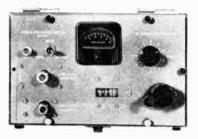
**FREQUENCY METER MODEL 802B** Range of 2350 to 10,500 megacycles covers the most used frequencies. Veeder-root digital counter provides accurate, legible readings which are referred to calibration charts for frequency in megacycles to rated accuracy of 0.2% without calculation. Completely self-contained with builtin detector and indicating meter.
