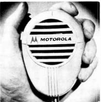
• Draws its power from the standard transmitter "talking current" supply, making it interchangeable with carbon microphones used with Motorola equipment.
