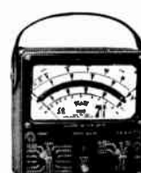
625-NA The First V-O-M With 10,000 Ohms/Volt AC
