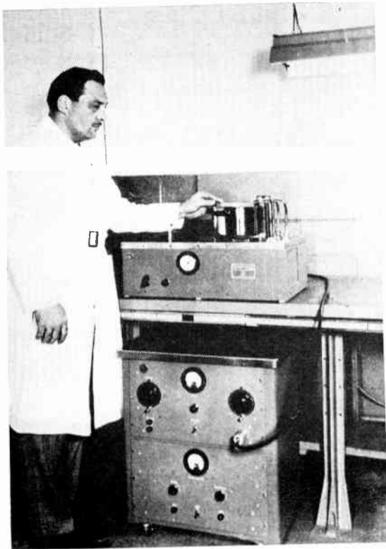
● This electrosonic cleaning equipment consists of two parts, a driver amplifier and a transducer with attached cleaning tank. The equipment is fully portable and can be easily moved from one section of a plant to another without trouble.
