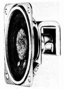
The Model 25A07 is only 1¼" deep, maximum input, 2 watts; 0.65 Alnico V magnet; U-shaped pot; impedance 3.2 ohms, 10%. For the replacement field it is supplied with four threaded mounting holes on the pot, in addition to the four rim mounting holes. Quam-Nichols Co., 240 East Marquette Road, Chicago 37, Illinois.
