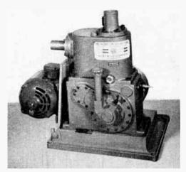
Only NRC Rotary Gas Ballast Pumps have proved, on thousands of installations, that they keep their original high efficiency even when pumping 100% moisture or other troublesome vapors. The reason is that only NRC pumps have been designed around the gas ballast principle, which, with other features, keeps vapors from condensing, keeps oil clean, maintains initial fast cycles day after day.
