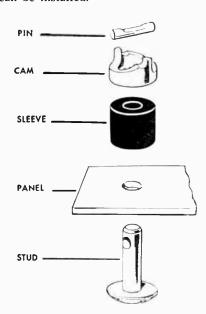
The Vibrex Fastener is mounted in a hole in the removable panel. The stud is inserted through the hole in the panel, rubber sleeeve, and cam, as in the diagram. To insert the pin in the stud, the cam is pressed down, slightly compressing the sleeve. This can be done by hand but special tools are available.
