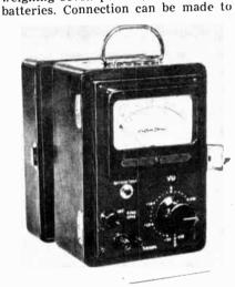
it through either binding posts or a telephone type jack and both bridging and terminating input impedances are available. Means are provided for checking the condition of the batteries and for adjusting the calibration.
