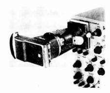
Speed and facility of mounting enables a single camera to service several scopes of various types and manufacture.
