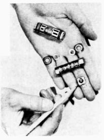
size photo. The cell itself, smaller than a fingertip, yet a third more powerful than conventional flat cells, is made entirely by machine and is sealed in an airtight pliofilm envelope. Merely stacking 15 such cells in a column wrapped tightly with transparent plastic and capping it in a leakproof tube of drawn aluminum produces this 22½ volt battery for pocket radios, hearing aids, Geiger counters, and other small electronic devices.
