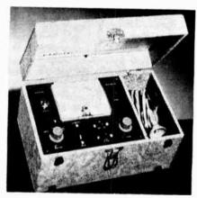
The Model CC-1 tests all electromagnetic deflection picture tubes normally encountered in television servicing. Supplies all operating voltages to the tube under test, and indicates the condition of the tube on a large "Good-Bad" scale. Features spring loaded test switches for operator protection.
