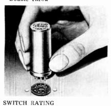
operations 24 volt non-inductive load Greater load capacity at fewer operations. CONTACTS Solid coined silver COIL RESISTANCE To 10,000 OHMS SHOCK TEST — 50 G VIBRATION Excellent characteristics due to small armature mass. INSULATION 500 volt any terminal to ground HERMETICALLY SEALED OPERATING TEMPERATURE -55°C— +85°C BASE TO FIT 7-PIN Miniature tube socket
