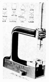
line of its kind, have announced a new product, the "HAM-R-PRESS". This precision punch is the easiest way to cut an exact, clean mounting hole for any electronic part — without drilling.
