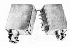
approximately 50-ohms impedance and generally satisfactory for frequencies up to 1,000 mc. Clamping parts, that require no soldering of the braid wires, are available in various sizes for coaxial cables from  $\frac{1}{16}$  OD up to  $\frac{1}{4}$  inch for RG-59/U etc. cables.
