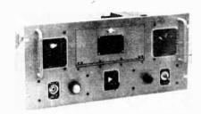
per cent distortion. Either tone or do signals are accepted by the TT-63A. The output may be polar or neutral signals. The Stelma TT-63A is being used throughout the U.S. Government Services.
