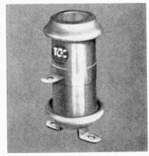
The glazed ceramic rim is designed to eliminate corona losses at the edges of the dielectric. The electrodes consist of substantial fired-on silver layers to which the terminals are soldered.
