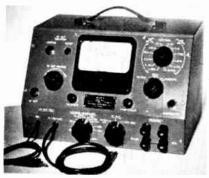
high-speed safety relay protects personnel from shock danger and a built in calibrator assures accuracy. Primary input measurement errors are eliminated because voltage is read directly across output leads. Highest voltage ranges are provided at slight extra cost.
