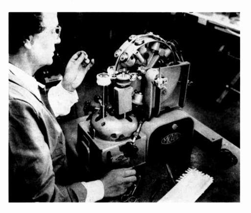
The Swiss-made MICAFIL RW-I Toroidal Coil Winding Machine in operation at Sperry Gyroscope Co. Ltd., Montreal, for precision winding of coils for the aircraft and electronics industry.
