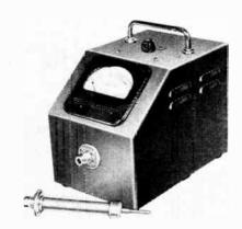
Thus in a single power meter a resistance of 50, 75 and 93 can be readily set providing a correct terminating resistance for each of the standard line impedances. For additional information refer to the display advertisement in this issue.
