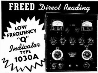
Measures the "Q" factor of coils directly and the inductance of coils, distributed capacity, impedance and dielectric losses. The "Q" Indicator can be used to study the magnetic properties of iron, such as stability of iron cores in function of applied voltages, and, iron losses as a function of the frequency.
