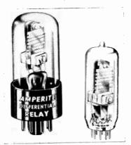
The Amperite Differential Relay is available in either the standard octal base or nine-pin miniature. They are pre-set at the factory. Standard tolerance of voltage or current for opening and closing is  $\pm 10$  per cent. Closer tolerances are available on special order. The Relay is compact, light, rugged. Being hermetically sealed, they are not affected by changes in temperature, pressure, or humidity. List price is \$4.00 each.
