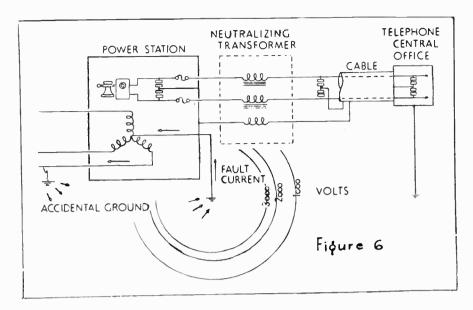
excessive exciting current may damage the primary winding. The secondary potential impressed on the terminal apparatus, may be very high depending on the frequency of the extraneous potential. Therefore, an insulating transformer does not offer satisfactory protection.
