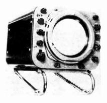
similar conditions preclude the use of Marine Radar, Decca 214 has an application. Range scales from 1/2 to 10 Kilowatts and a pulse length of 0.05 u.sec. with receiver band width of 20 m.c/s ensures high definition with a range discrimination of 10 yards.
