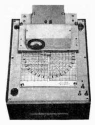
ink recorders plot ac or dc electrical voltage levels in either polar or rectangular co-ordinates on linear, square root, or decibel scales.
