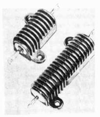
maximum heat resistance, and are impervious to moisture. The RH's are further sealed in a die-cast, black anodized radiator finned housing. Temperature coefficient is 0.00002/Degree C; resistance ranges are from 0.1 ohm to 55,000 ohms depending on type; tolerances are from 0.05% to 5%.
