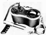
Engineered for rugged field use, all sensitive and delicate electronic components have been shock mounted and protected by non-breakable casing and high grade aluminum. Waterproof seals and ruggedized hermetically sealed meter enable this instrument to be used under the most adverse climatic conditions.
