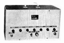
duces new type of wave form for "go, no-go" indications. Three  $\sin^2$  pulse widths are provided: 0.25, 0.125 and 0.062 usec corresponding to bandwidths of 2MC, 4MC and 8MC, respectively. Size, 8 x  $15\frac{1}{2}$  in.
