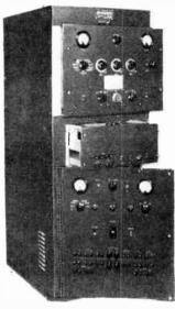
acceptable R/T service. The transmitter will deliver better than 1000 watts into a 50-75 ohm transmission line, and is continuously tunable over a frequency range of 200-530 kcs. All tuning controls are located on the front panel of the transmitter, and operating
