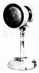
The sensitivity naturally varies with the type of aircraft transmitter used, but bearings obtained are accurate to distances as great as those at which voice communication can be maintained between the tower and the aircraft.
