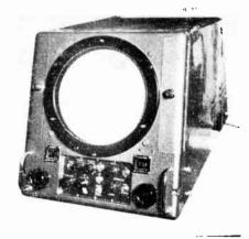
minimum of time and expense. The Decea Universal Display incorporates a fixed coil design allowing several interscans and considerable flexibility in the type of presentation. Unit chassis of the "plug-in" type contain the various deflection, gating, calibration, mixing and interscan circuits and these individual chassis can be readily changed to alter the function of the display. The viewing unit itself is
