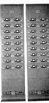
Multi Channel Frequency Modulated Telegraph Systems capable of multiplexing such circuits as telephone lines, V.H.F., U.H.F., or Radio Frequency Links, designed to meet any speed requirements, fully electronic, without relays or moving parts to wear.
