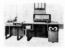
Plotter features numeric abscissa printing. This provides for numeric printed identification of reference points along the lower edge of the plot. Characters may be printed at a
