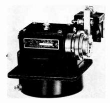
Model KBA synchronous motors are salient pole (phonic wheel) variable reluctance motors. The design employing a sixty-pole rotor limits the instantaneous angular shaft error caused by load or voltage changes to  $\pm 0.1$  degree. The windings will carry 80 m continuous duty. The voltage across the winding will vary with frequency; the upper limit for the applied voltage is 1000 y rms continuous duty.
