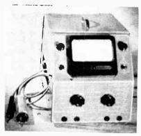
clarify much of the confusion in terms used in electronics today. The unit operates from 115 volts 60 cycles, and comes complete with test leads and high frequency probe.
