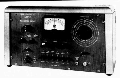
The Baird Associates Transistor Test Set is a versatile precision instrument designed to analyze transistors at any frequency from 100 cps to 1 mc in terms of well-known standard parameters. The transistor coefficients thus obtained enable the circuit designer to predict the performance of amplifiers in the AUDIO, INTERMEDIATE and LOW RADIO FREQUENCY ranges. Technical Circular \*\*RD 511-A.
