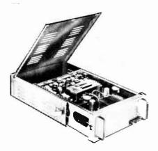
The 6000 series mobile transmitter and receiver may be supplied and equipped for two frequency operation within a spread of 300 Kc. Universal 6/12 volt operation is accomplished automatically by the battery connector. No wiring changes are required.
