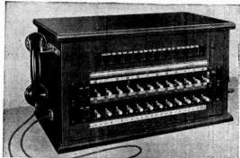
Cordless Switchboards, both C. B. and Magneto
