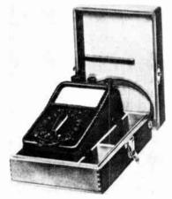
ranges (3 ma to 1.5 amperes); 5 resistance ranges (100 ohms to 100 megohms) and a capacitance range (0.005  $\mu f$  to 10  $\mu f$ ). Accuracy is  $\pm$  1.5% on D.C. and  $\pm$  2.5% on A.C. Meter is color coded and operating instructions are printed on back. Meter is dust- and moisture-proof.
