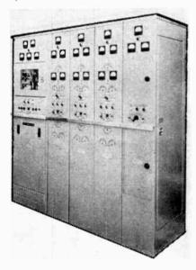
Unitized construction is employed with separate rectifier and RF units, providing maximum flexibility. A unique feature is the absence of conventional tuning elements in the LF/MF units. These components are replaced by specially designed Hipersil cored transformers.
