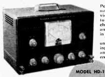
Performs the functions of more elaborate and much more expensive audio distortion testing devices and yet is simple to operate and inexpensive to own. Used with a sine wave generator, it will check the harmonic distortion output of audio amplifiers under a variety of conditions. Essential in audio design work.
