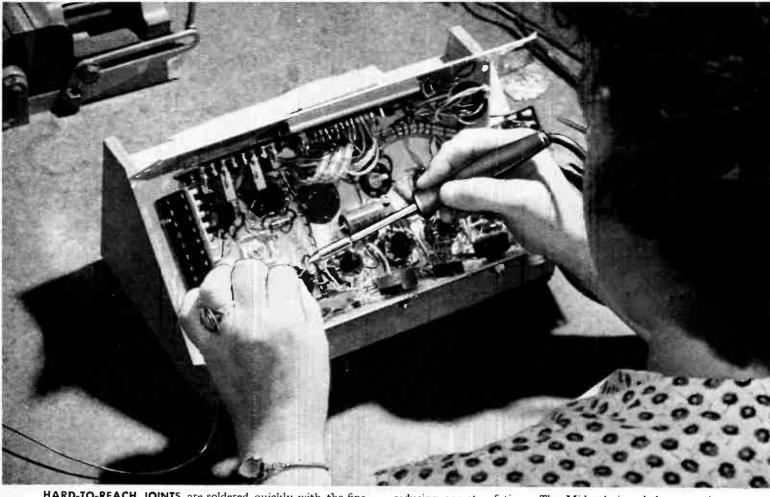
**HARD-TO-REACH JOINTS** are soldered quickly with the fine-point G-E Midget iron—with no damage to adjacent parts. Weight of iron—less than 3 ounces—helps increase output by
