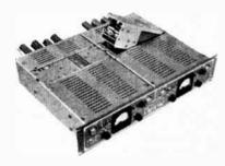
The Northern Radio Dual Frequency Shift Tone Converter achieves great simplicity by utilizing a new pulse type discriminator. The discrimination of mark and space frequencies can be made within three cycles. This discriminator, coupled with a high degree of limiting permits a minimum of systems distortion and a maximum of noise interference rejection.
