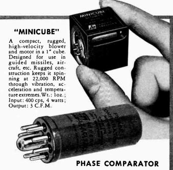
A versatile, full wave bridge comparator for use as a modulator, demodulator, or switch. Frequency Response: 0-5000 cps; Max. Reference Voltage: 120 V. rms; Max. Output Voltages: ±50 V. DC; Dynamic Range: 46 db. Hermetically sealed.
