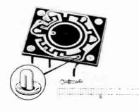
Grove, N.Y. Note how the wired plugs enter through set-in eyelets and lock automatically (inset shows contact magnified.) Plug can easily be disconnected, yet never disconnects accidentally.
