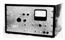
through the feedback resistor. Voltage output is therefore equal to feedback resistance is therefore equal to feedback resistance multiplied by input current. Current gain is substantially independent of the amplifier gain and is therefore independent of the characteristics of the amplifier tubes. Dynamic input resistance rises from 2500 ohm on the 10-7 amp range to 25,000 megohm on the 10-11 range.
