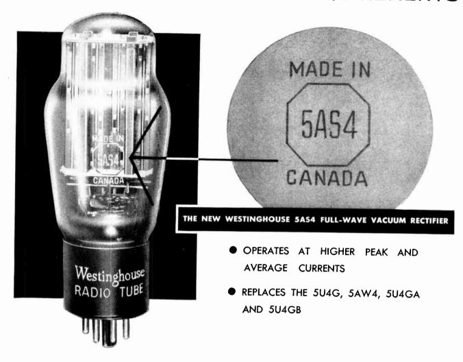
Modern, large-screen TV receivers require high DC power output. To meet this need, Canadian Westinghouse has designed the 5AS4 . . . completely engineered in Canada for the Canadian Television Industry. The Westinghouse 5AS4 has new plate, cathode and mount designs. The large mount structure, enclosed in an ST-16 envelope provides for more uniform heat distribution and permits operation of the tube at higher peak and average currents than the prototype 5U4G.
