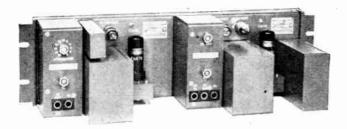
A send and a receive panel require  $5 \% ^{\prime\prime}$  of mounting space on a standard  $19 ^{\prime\prime}$  rack
