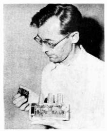
Comparison of transistor and conventional tube circuit.
