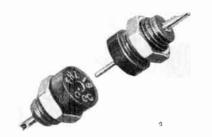
The extremely rugged "FHL" has high dielectric characteristics and features the use of one-piece moldings available in three in-sulating materials: Mineral (asbestos) filled Melamine for high dielectric and mechanical strength, Plaskon Reinforced (glass) Aklyd type 440A for unusually high impact strength and arc resistance, and Diallyl Phthalate (blue) with high dimensional stability plus excellent dielectric properties. Precision-machined socket and pin contacts
