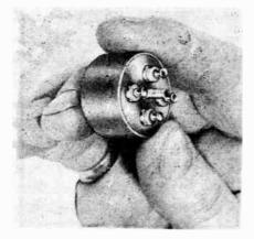
weighs but 1½ oz. Electrical ratings are: Input, 115 volts, 400 cycles; Power output, 6 VA; Regulation, 10 per cent; Heat rise 40°C, Class "A". It is hermetically sealed in a metal case to MIL-T-27 requirements.
