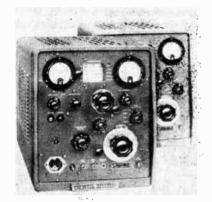
lightweight aluminum castings, ball bearing condenser and turret drives, sealed transformers, militarized construction, and special electrically welded - hp - condensers of low temperature coefficient Invar steel plates.
