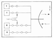
• Figure 1. Block diagram of two transmitters and two receivers diplexed over a common antenna by the use of tuned cavity directional filters.
