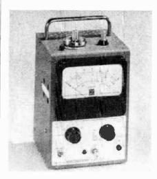
All Keithley Electrometer accessories fit the new model. It can thus be used not only as a dc voltmete, but as on extremely sensitive micromicroammeter, megohmm+ter, and Kilovoltmeter. Maximum full-scale sensitivities are 8 x 10<sup>-13</sup> ampere. 3 x 10<sup>11</sup> ohms, and 20.000 volts.
