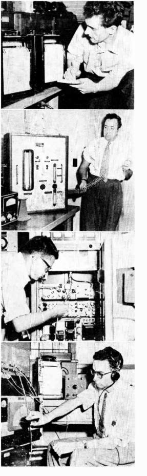
• Top: Collecting data in microwave section. Second from top: Measuring microwave power by heating water. Third from top: High frequency transmitter in RPL mobile lab. Bottom: Equipment used by the laboratory for ionosphere investigations.
