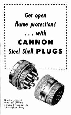
Use Cannon Steel Shell Firewall Connectors, in "AN" or "K" line. They effectively block the fire path at bulkheads by preventing passage of open flame through the connector assemblies at the firewall. Standard units in aircraft ... many industrial applications. Front and rear insulators are available in glass-filled material.
