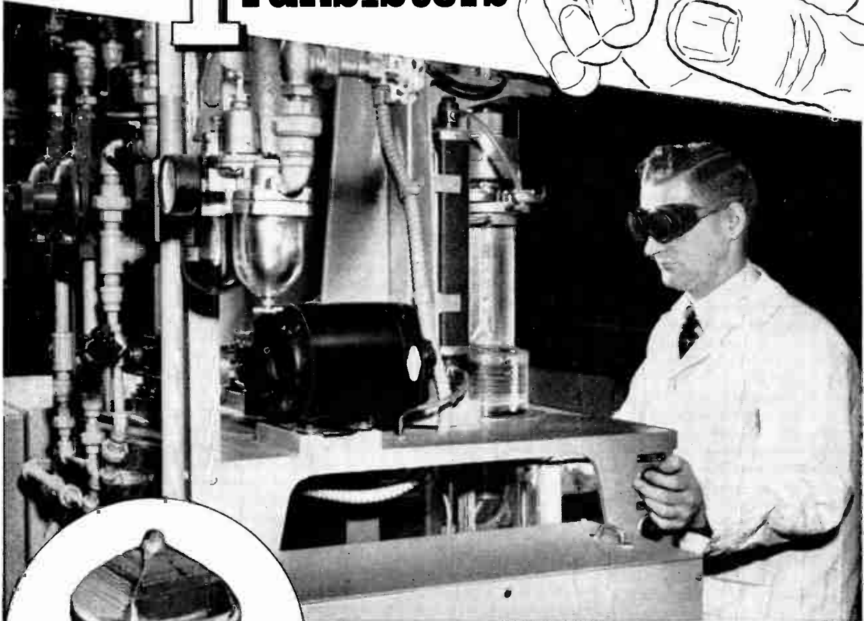
Skill is required to operate complicated equipment installed in our Montreal Plant to produce grown NPN crystals for Junction Transistors.
