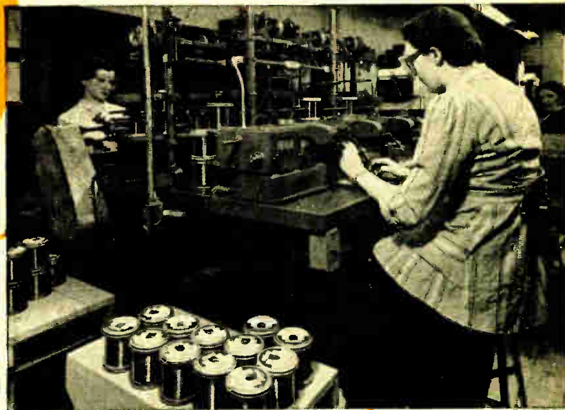
Winding relay coils with Phillips Enamel Magnet Wire.
