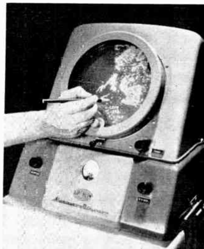
● REFLECTION PLOTTER is part of the new Model 1500 "Mariners Pathfinder" radar for small vessels.
