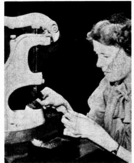
● Fig. 4—The platinum whisker wire is crimped to the required length and form in this press.
