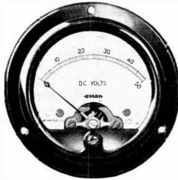
MODEL 604R. DC volts, amperes, milli-amperes, microamperes. Moulded bakelite 3½" round case, flush mounting, spade or lance type pointer. Scale length 2.4". Also available in 2½" round case—Model 605R.
