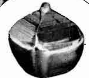
"Single crystal" of pure germanium grown in our plant for use in Junction Transistors.
