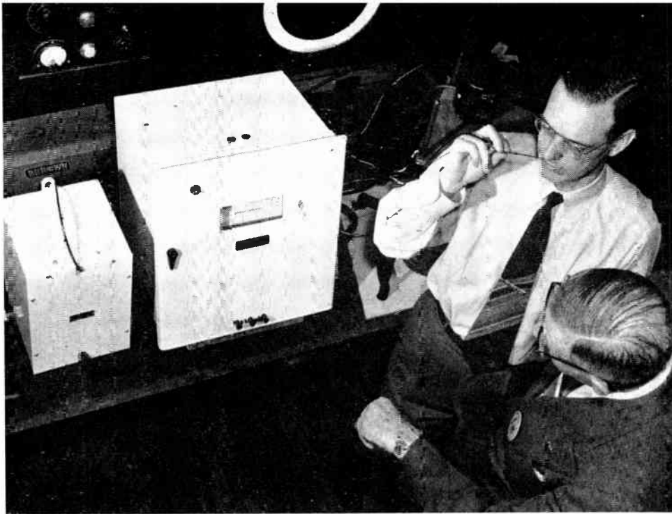
● To speed processing time of blood donors, engineers from Minneapolis-Honeywell's Industrial Division developed the "thermotron," shown above, an electronic instrument twice as accurate as a doctor's thermometer and 60 times as fast.
