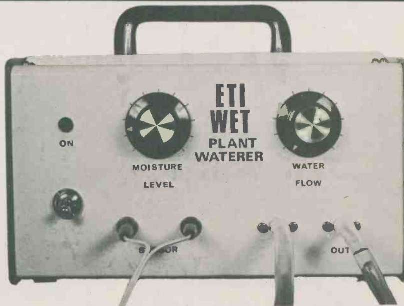
Head on view of the complete prototype, the LED can be left out if you want extended battery life.
