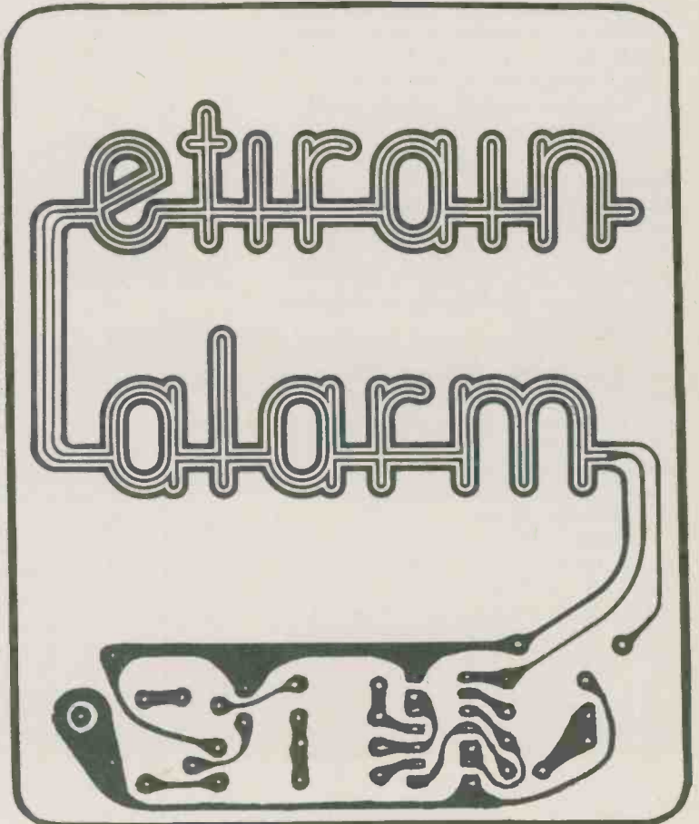
Fig. 4. Overlay of the section of the Rain Alarm PCB that holds the components.
