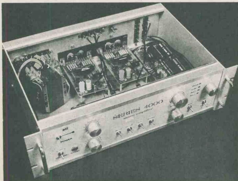
The complete stereo amplifier is shown here mounted in a handsome rack-mounting case.
