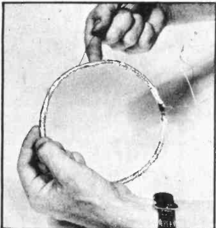
3: Wind tinned copper wire over the shield, passing the end out where the coil leads pass out.
