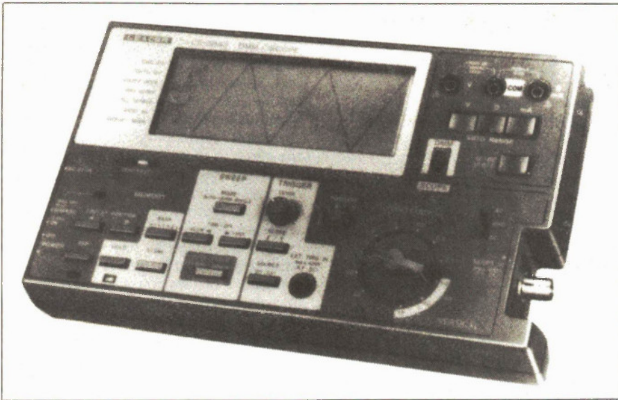
Fig. 6. The Leader LCD-5840 portable storage scope.
