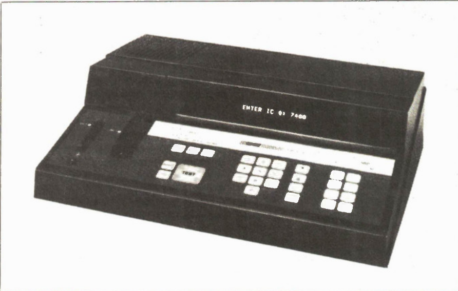
Fig. 7. The BK-Precision Model 560 programmable IC tester.
