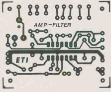
PCB for the DAC/ADC filter amplifier.
