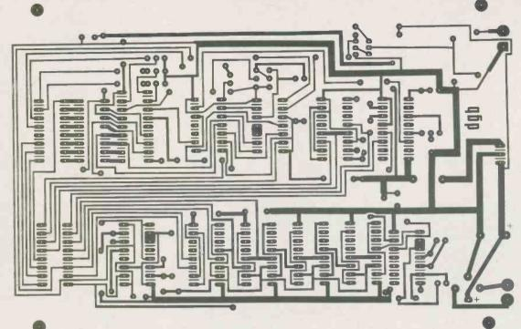
The printed circuit layouts for the main board and display.
