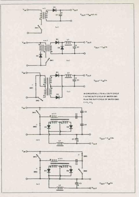
Fig. 3. Transformer-coupled switching mode circuits. (a) Flyback converter. (b) Single ended forward conver. (c) Push-pull converter. (d) Half bridge circuit. (e) Full bridge circuit.
