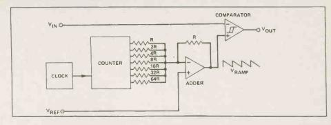
Fig. 3. Simplified block diagram of a simple A-to-D converter, the 507C.  $V_{REF}$  is an on-chip or external reference voltage.  $V_{IN}$  is analogue voltage to the converted;  $V_{OUT}$  is the square wave output.
