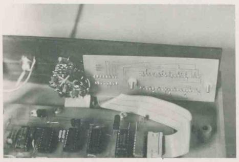
Figure 2. The display board.
