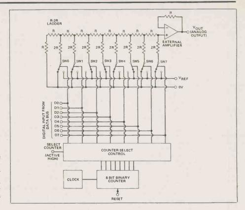
Fig. 5. Block diagram of the ZN425E D-to-A converter. V<sub>REF</sub> is an on-chip or external reference voltage. The amplifier is not on the chip, but is an external op-amp (eg. 741).
