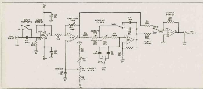
Fig. 1 Circuit diagram of the filter-amplifier.
