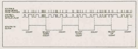
Fig. 3. Timing diagram of the circuit.
