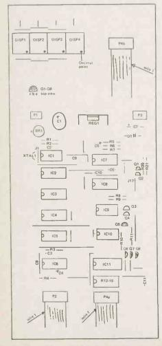
Parts overlay for the frequency counter.
