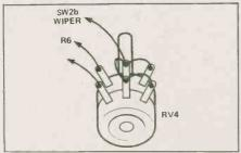
Fig. 2 (below) Connections to RV4
