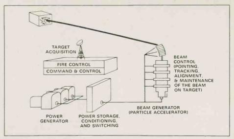
The basic layout of a particle beam weapons system.
