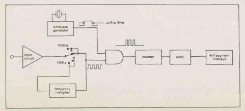
Figure 1. Frequency counter block diagram.
