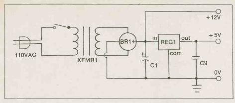
Power supply schematic for the frequency counter.
