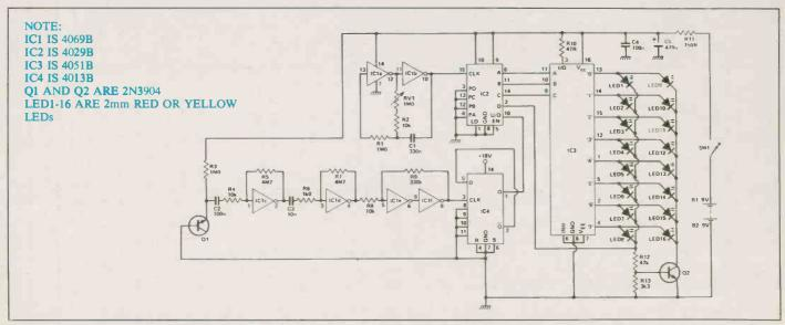
Fig. 2. Circuit diagram of the Infinite Improbability Detector.
