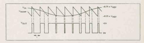
Fig. 4. The input and output voltages of the 507C A-to-D converter. The computer measures t, which is proportional to  $V_{\rm IN}$ .
