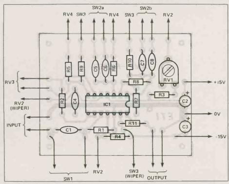
Component overlay for the PCB.
