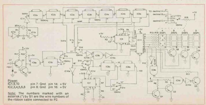
Schematic diagram for the frequency counter.
