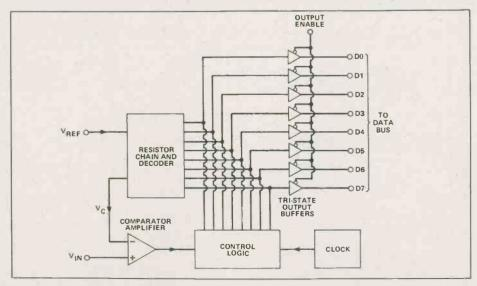
Fig. 2. Simplified block diagram of an A-to-D converter such as the ADC0801.  $V_{REF}$  is an onchip or external reference voltage.  $V_{C}$  is the output voltage from the resistor chain, which is compared with  $V_{IN}$ , the analogue voltage which is to be converted.
