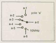
each pole is operational; this may save considerable time if troubleshooting is required later. Use table 1 to connect an eleven inch piece of ribbon cable to the switch.
