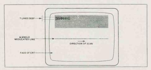
Fig. 6. How text is displayed on a TV screen.
