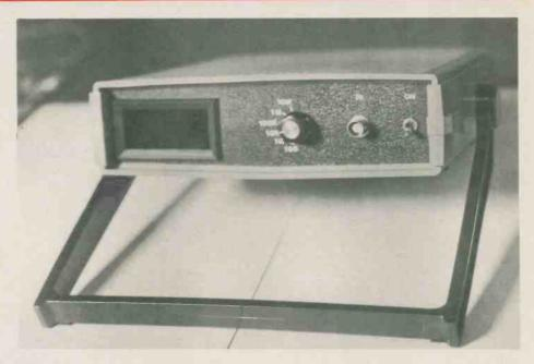
This frequency counter automatically updates its display about three times every second (approximately once per second on the 100 Hz range), and a latch is used to provide a flicker-free display of the input frequency.
