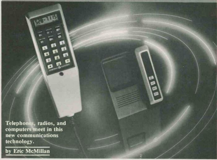
A portable handset unit for cellular radio, offered by GE/Northern Telecom. Photo courtesy General Electric.
