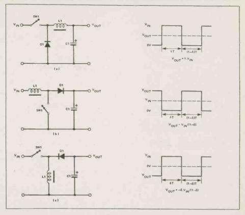
Fig 2. Circuit configurations to achieve different  $V_{\rm in}/V_{\rm OUT}$  (a) Voltage step-down. (b) Voltage step-up. (c) Voltage inversion.
